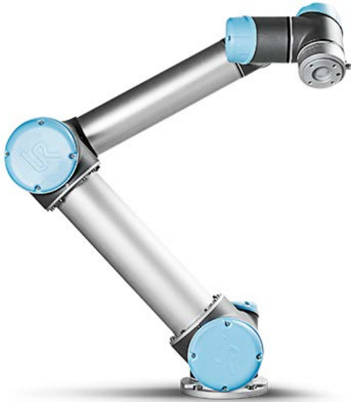
Figure 3-4 UR5 robotic arm for handling the arc torch
