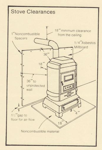
transferred from the stove to the floor. Be certain that both floor and wall protection extend far enough for adequate protection when a stove or Franklin type fireplace is set on a hearth or inside a stone or brick fireplace.
