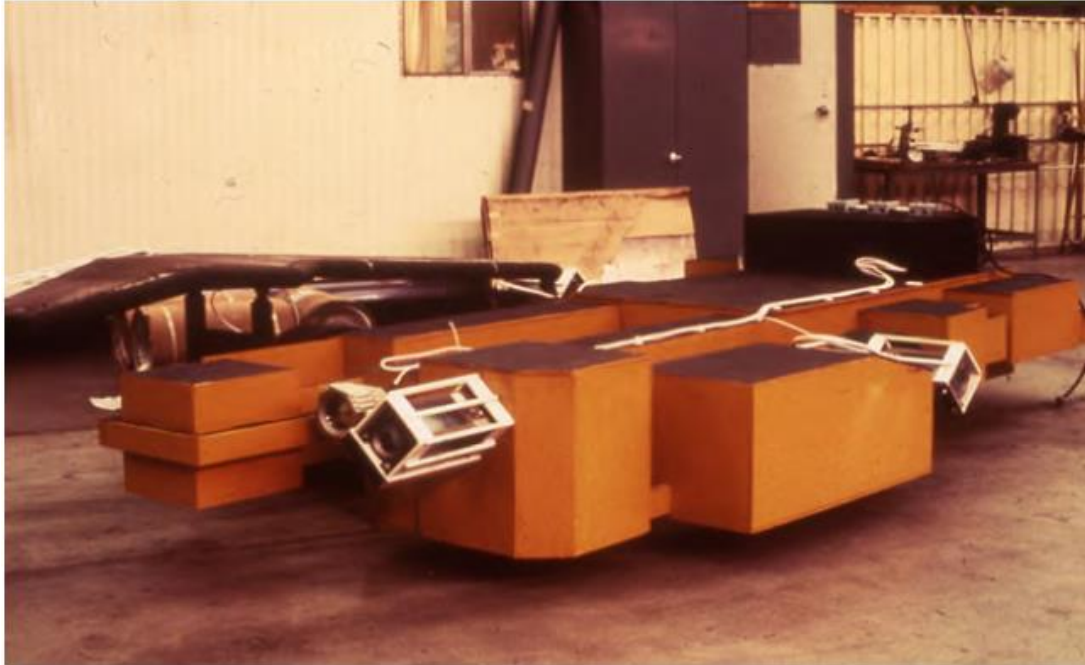
Figure 2.7: Wooden Mockup Used by USBM to Evaluate Machine Mounted Lighting (Sammarco and Carr, 2010)
