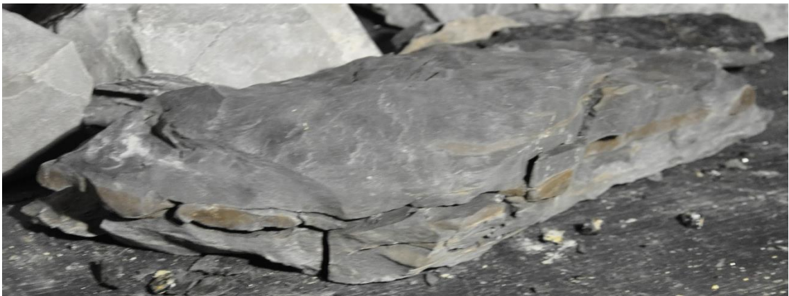
Figure 4.37: Fractured Shale Using HID Horizontal Flood Beam Pattern
