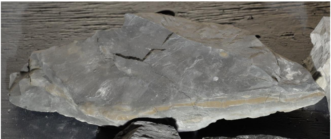
Figure 4.16: Shale Microfracture Using HID Horizontal Flood Beam Pattern
