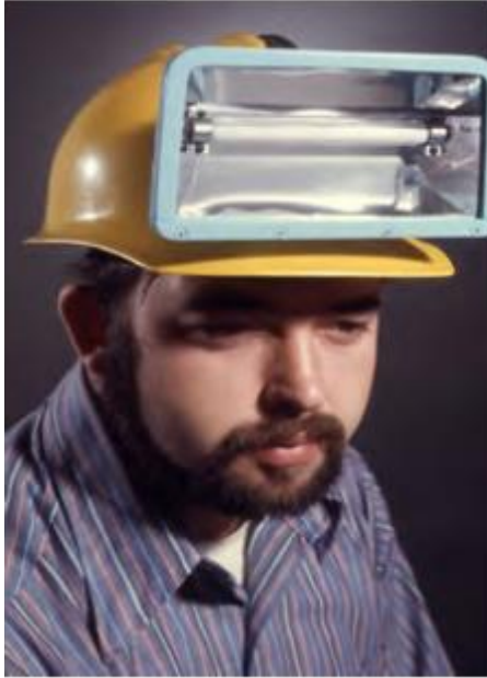
Figure 2.6: Fluorescent Cap Lamp (Sammarco and Carr, 2010)
