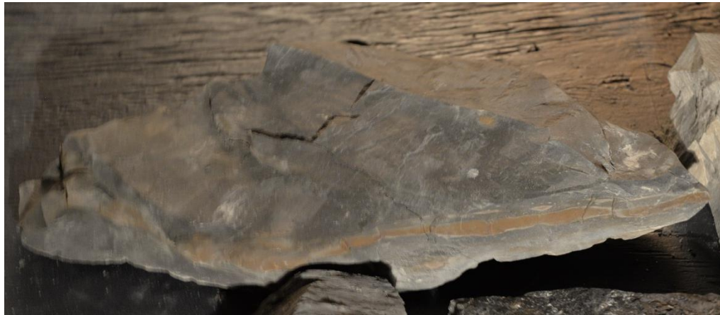
Figure 4.10: Shale Microfracture Using Halogen Euro Beam Pattern
