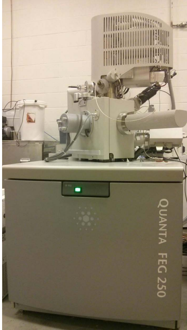
Figure 4-7: An Environmental Scanning Electron Microscope (ESEM) supplied by FEI.
