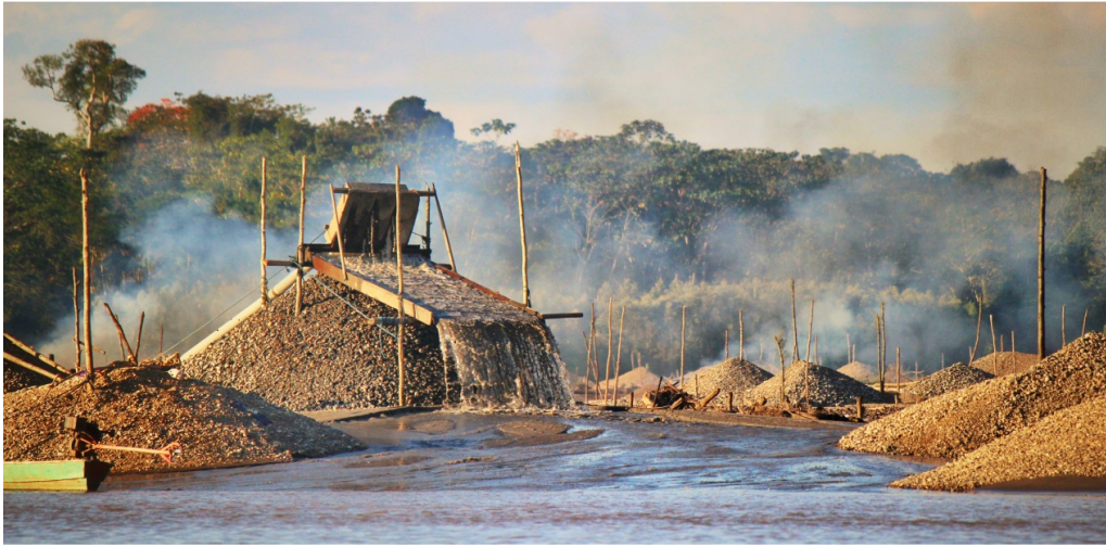
Figure 1. Caranchera (semi-mechanized mining machine) on the Madre de Dios River in Peru
