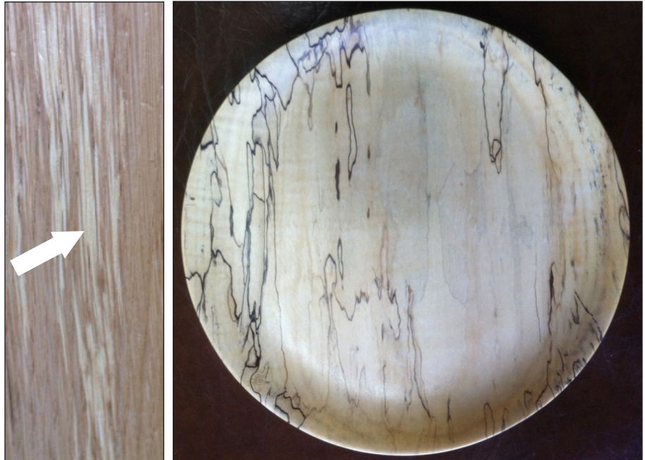
Figure 2-5. Two different pieces of wood in the initial stages of decay (“incipient decay”). The piece on the left is white oak, and the lighter patches (indicated by the arrow) are caused by a fungal infection. The plate on the right is turned from a piece of spalted red maple, and there are multiple black zone lines present.
