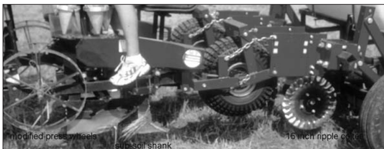
Figure 3. Modifications to a transplanter for no-till transplanting of tobacco.
