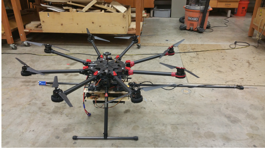
Figure 4.2: BLUECAT4 multi-rotor equipped with hot-wire instrumentation.
