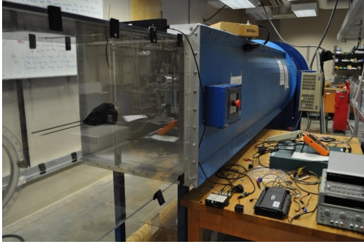
Figure 4.3: BLUECAT3 nose cone in wind tunnel during wind tunnel tests for BLUECAT3 instrumentation.
