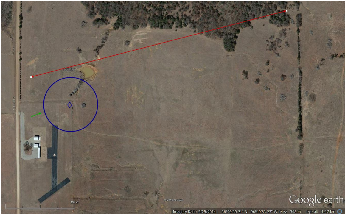
Figure 5.8: Oklahoma State's Unmanned Aircraft Flight Station with day one experiment's flight paths. Blue circle: BC5A flight path; Red Line: BC5B flight path; Blue diamond: Sonic anemometer; Green arrow: takeoff location and direction.
