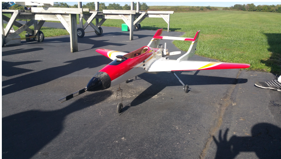
Figure 4.1: BLUECAT3 airframe equipped with hot-wire instrumentation.
