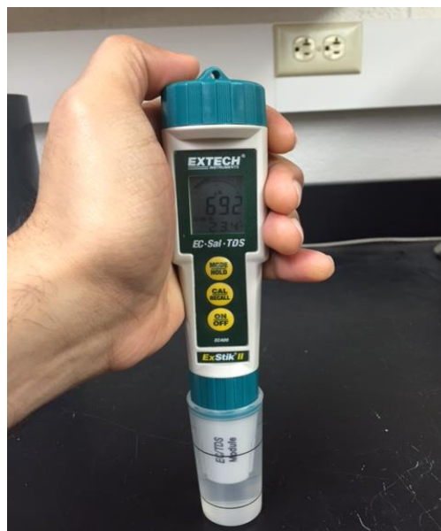
Figure 3.15. Measuring pore-water resistivity using Extech-400 conductivity meter
