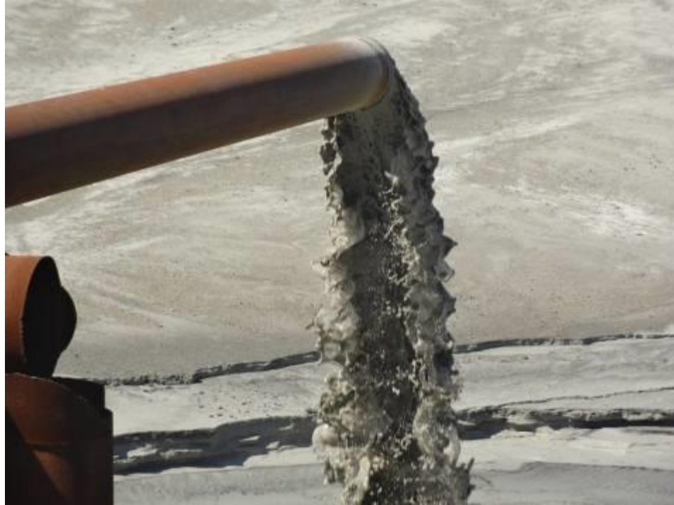
Figure 1.2: Wet disposal method
