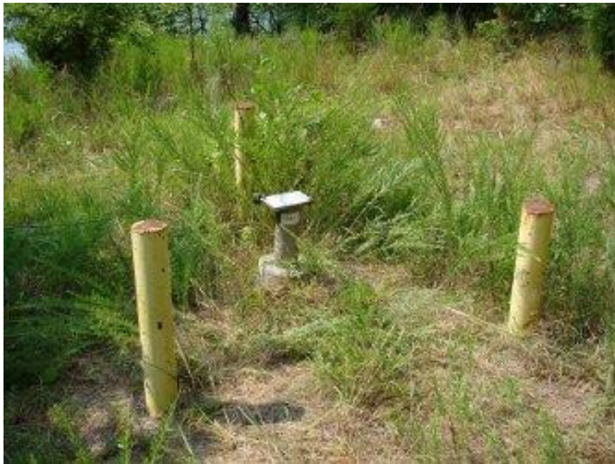
Figure 1.7: Groundwater monitoring well
