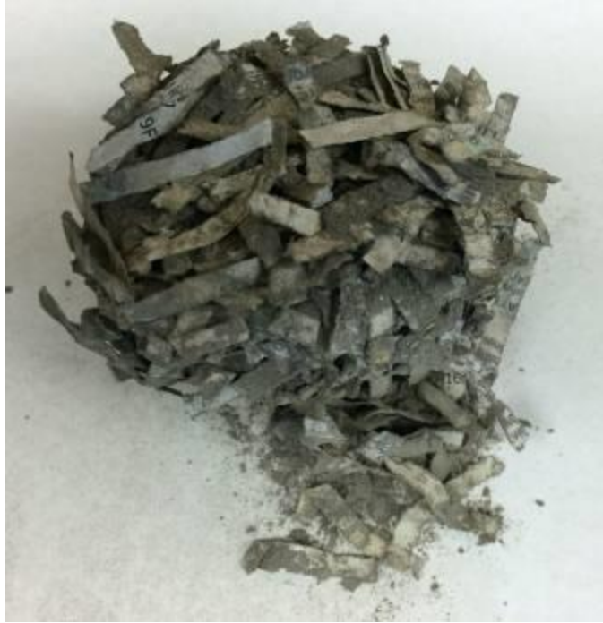
Figure 4.8: 80% Fly ash Class F and 20 % shredded paper
