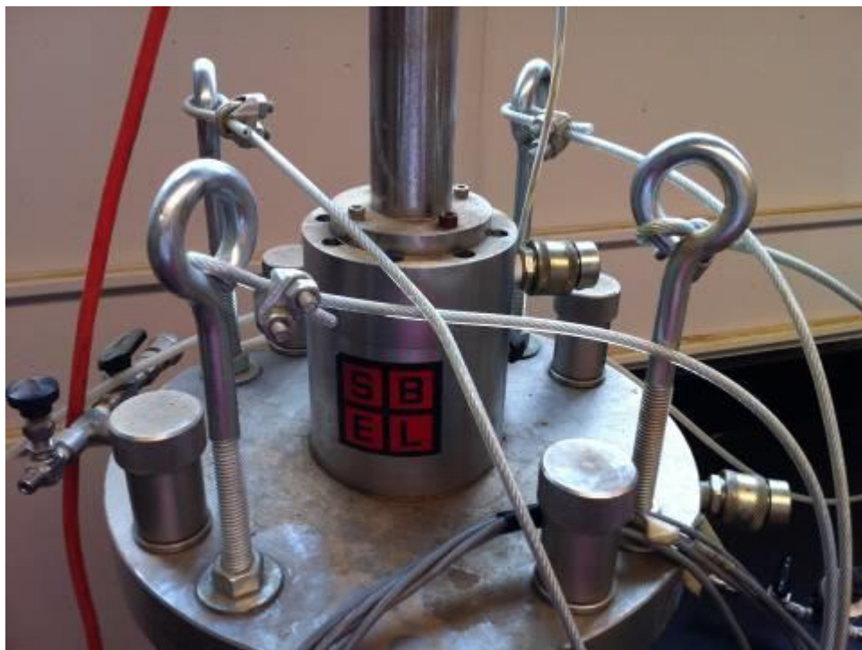
Figure B.9: Four washers and four nuts on top platen
