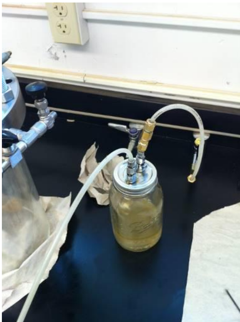
Figure B.6: Vacuum water trap
