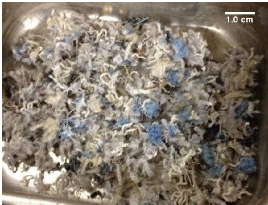
Figure 2.7: Shredded carpet after hand shredding
