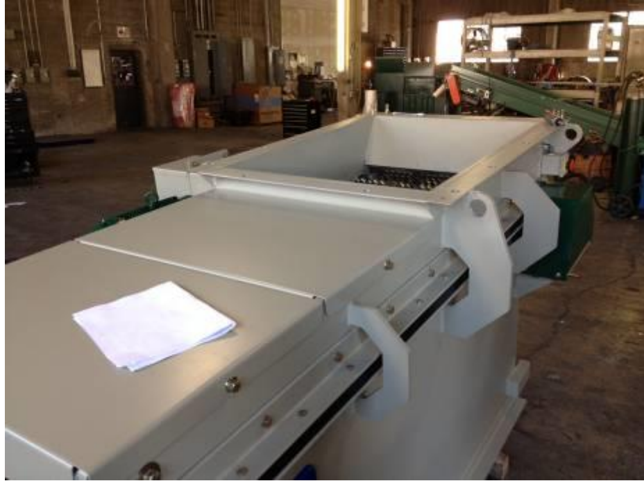
Figure 2.5: Carpet Shredder machinery
