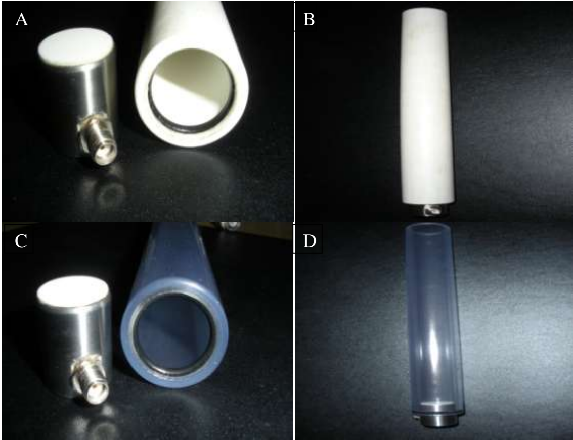
Figure 14. Acoustic Monitoring Tubes and Sensors. (A) White monitoring tube with view of o-ring placement and model R6 \alpha sensor, (B) White monitoring tube with R6 \alpha sensor fully inserted, (C) Clear monitoring tube with view of o-ring placement and R6 \alpha sensor and (D) Clear monitoring tube with R6 \alpha sensor fully inserted.
