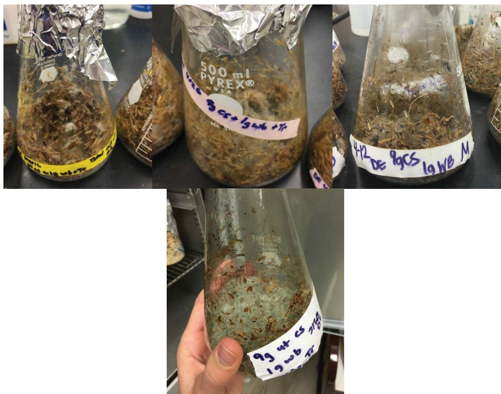
Pictures of samples with nine grams of corn stover and one gram of wheat bran after seven days. The sample on the top left was pretreated while the others were not.
