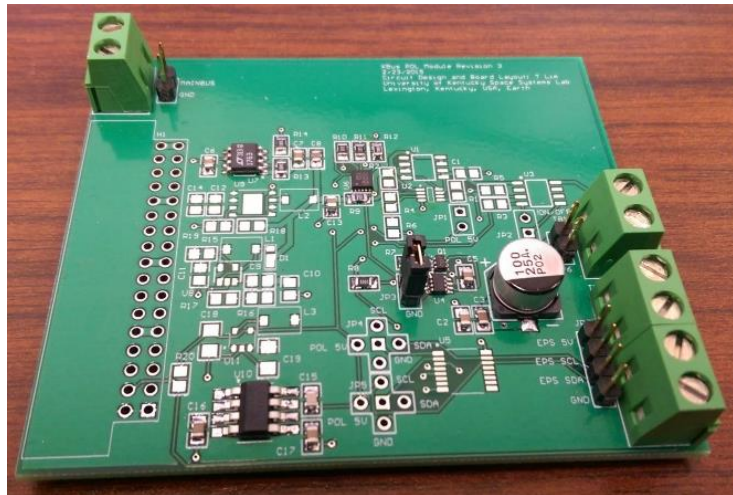
Figure 21: Payload Module Prototype
