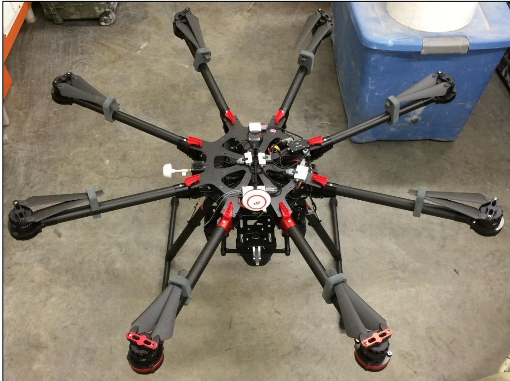
Figure 4.2: DJI S1000+ Equipped with Flight Electronics
