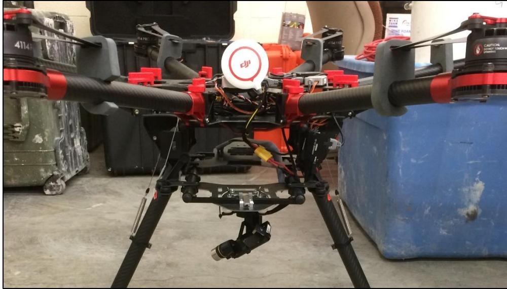
Figure 4.3: Battery Tray With Gimbal Attachment Below
