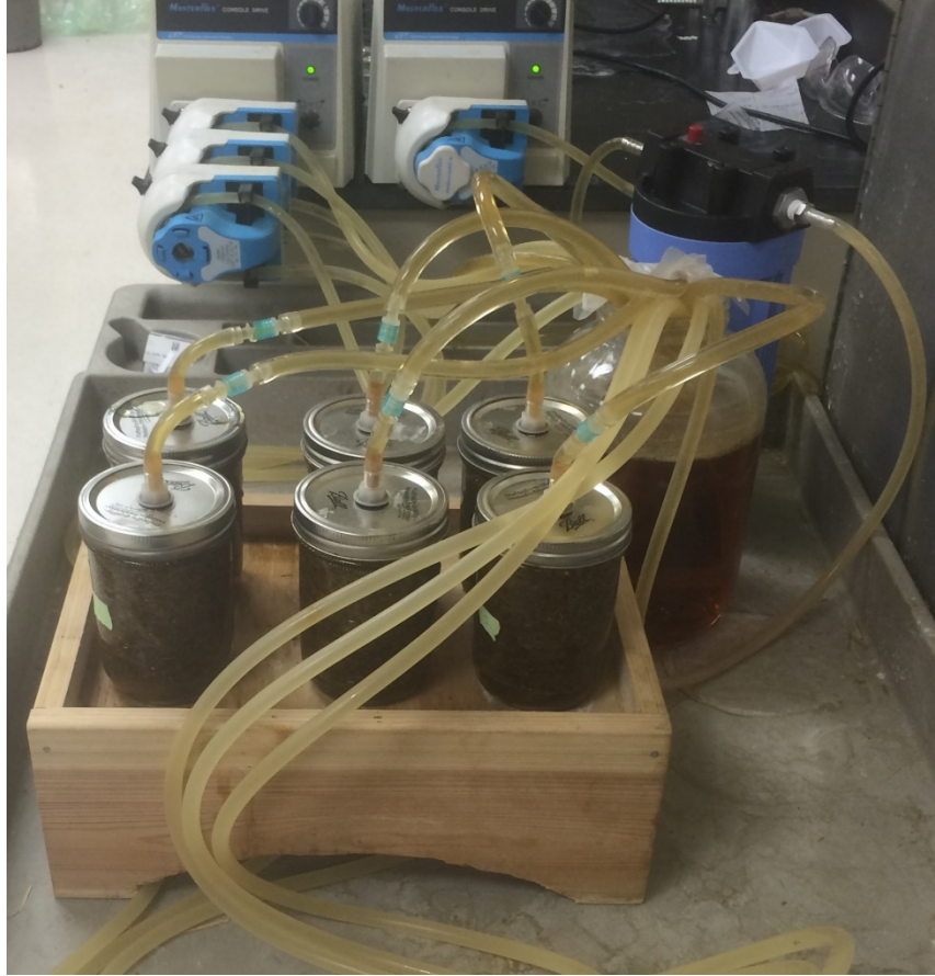
Figure 4: Experimental Pretreatment System
