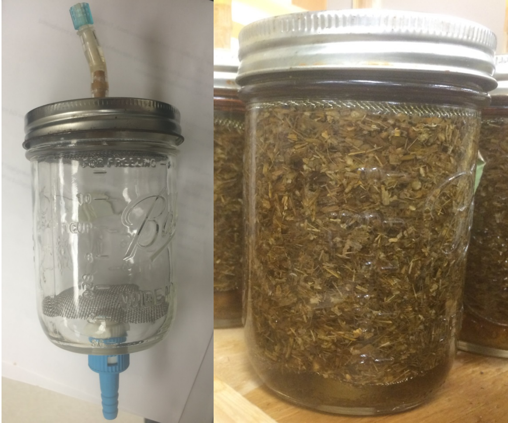
Figure 8: Up-flow Treatment Vessel left; Vessel with 38 gDM right
