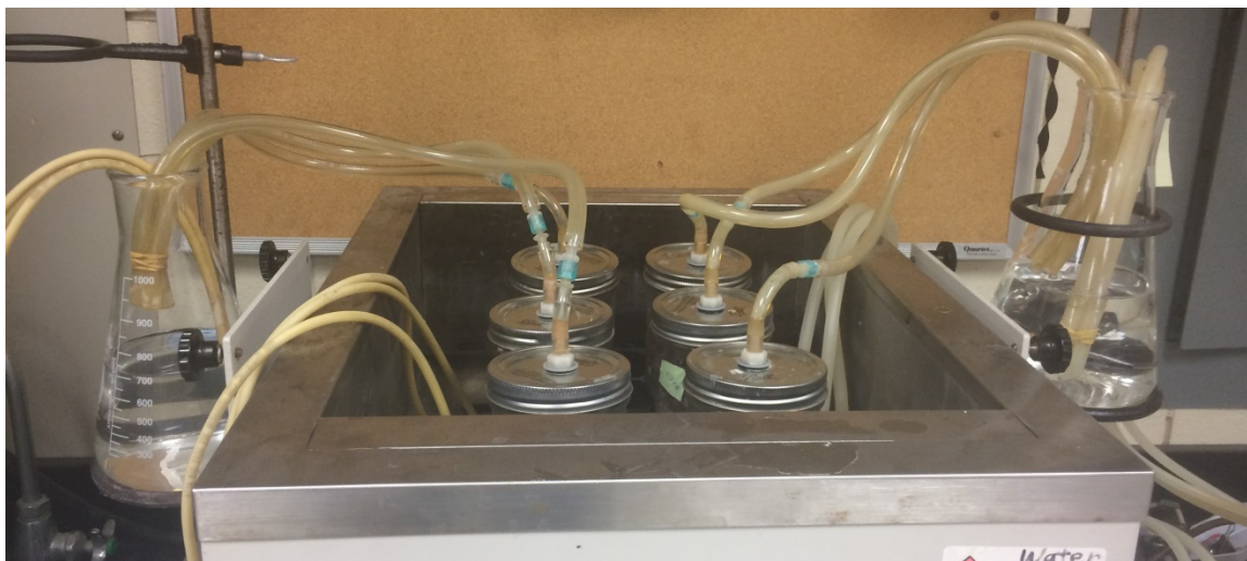
Figure 11: Experimental Bulk Enzymatic Hydrolysis System
