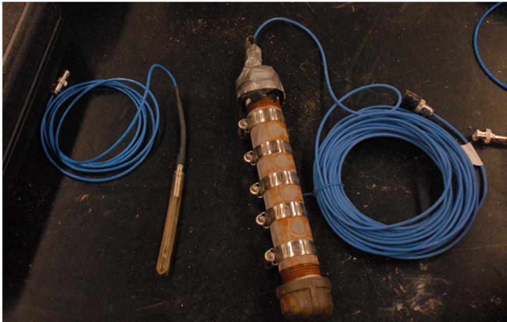
Figure 22: Uncased PCB tourmaline sensor (left) and cased PCB tourmaline sensor (right)
