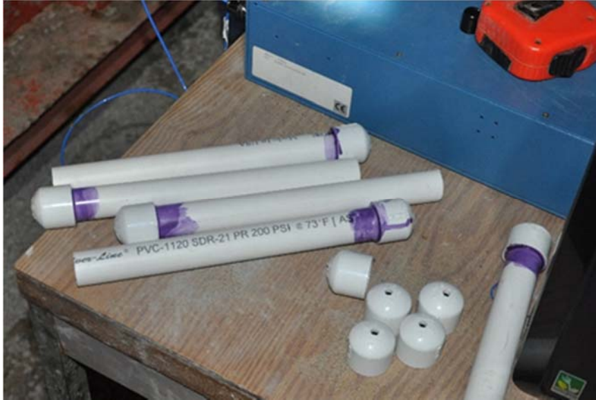
Figure 28: PVC pipe solution for charge burial in saturated conditions.
