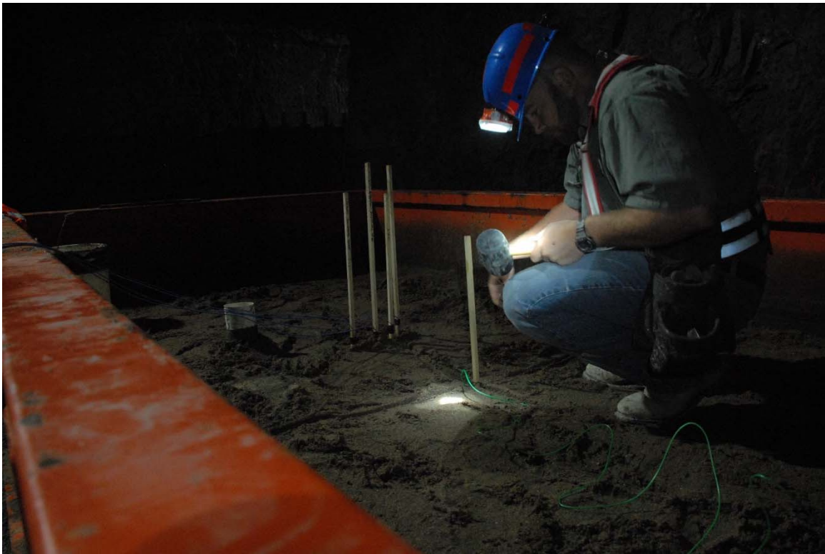
Figure 29: Test setup with wooden rods for charge burial and sensor measurements featuring Dr. Braden Lusk.
