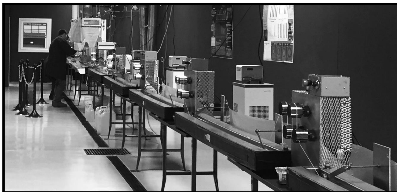
Figure 2. Solution spinning line at the University of Kentucky Center for Applied Energy Research (UKY CAER).
