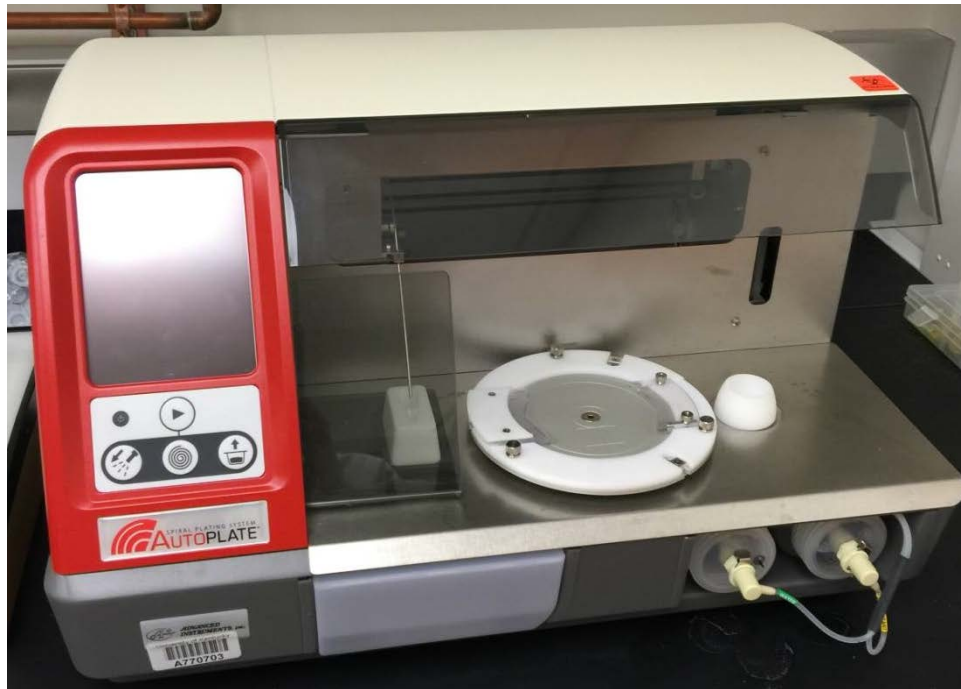
Figure 3.16: AutoPlate ® spiral plater; Advanced Instruments, Inc., Norwood, MA
