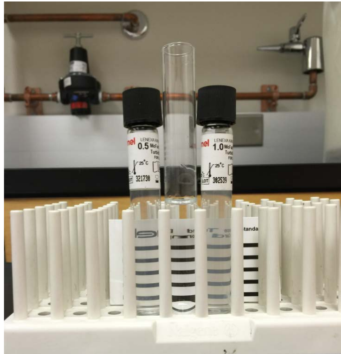
Figure 3.8: Test Tube with Water, McFarland Standards and Wickerham Card
