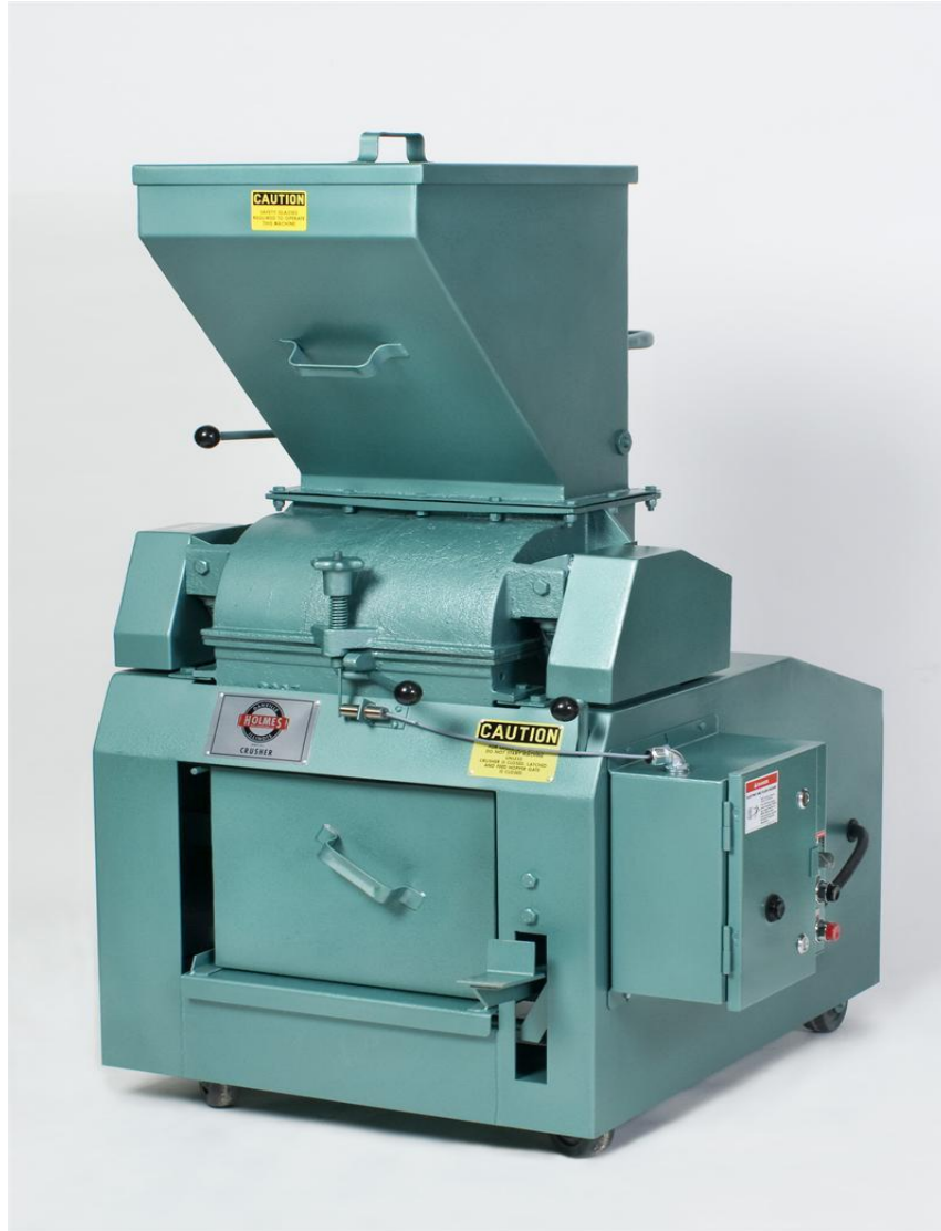
Figure 4-2: Holmes model 401XL Hammer Mill Coal Crusher (courtesy of Preiser Scientific)
