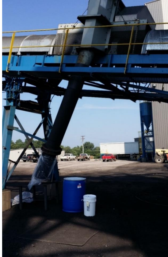
Figure 4-1: Sample collection from clean coal product of Dense Medium Cyclone
