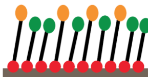
Figure 1.4. Schematic presentation of a mixed self-assembled monolayer consisting of two different adsorbates with different chain length and terminal functional group.
