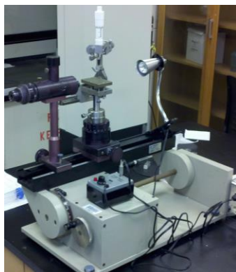
Figure 2.2. Photograph of Goniometer used for all the measurements [108].
