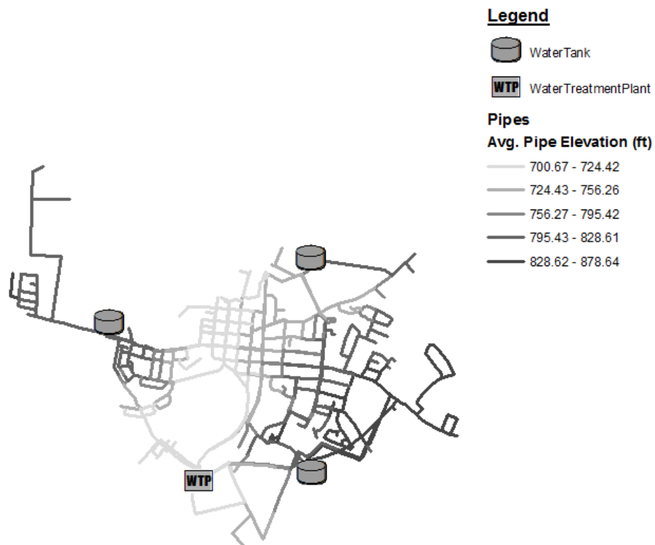
Figure C.98: Average Pipe Elevation for KY14.
