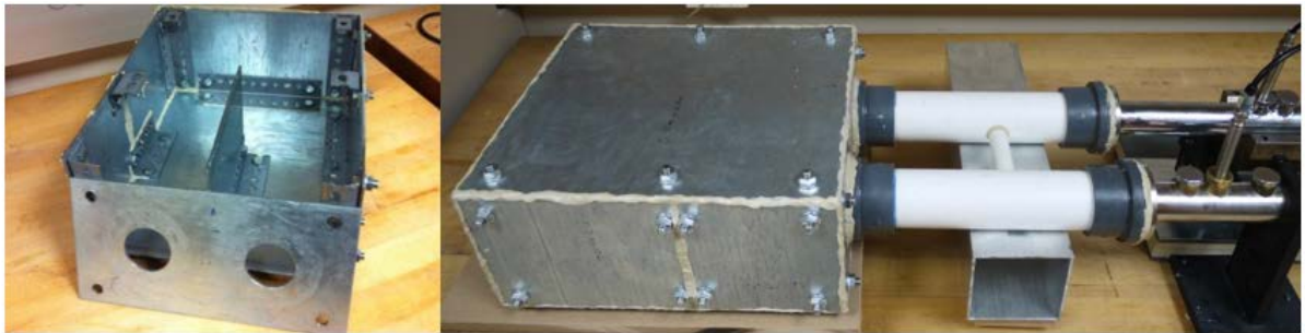
Figure 4.9 The experimental muffler with and without bypass duct.
