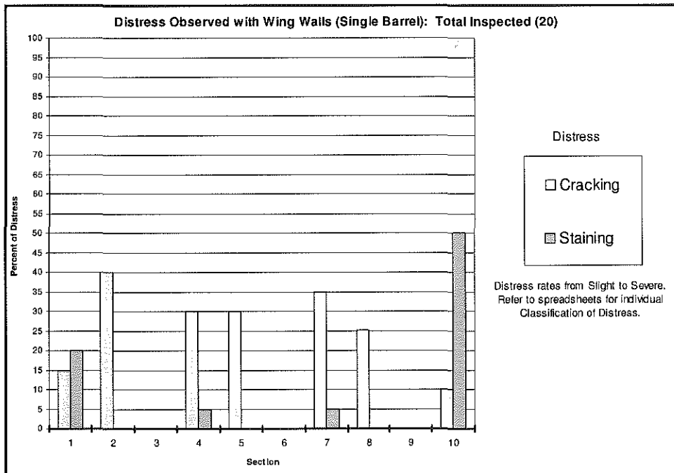
Figure 25: Distress Observed in Culvert Wing Walls (Single Barrel)
