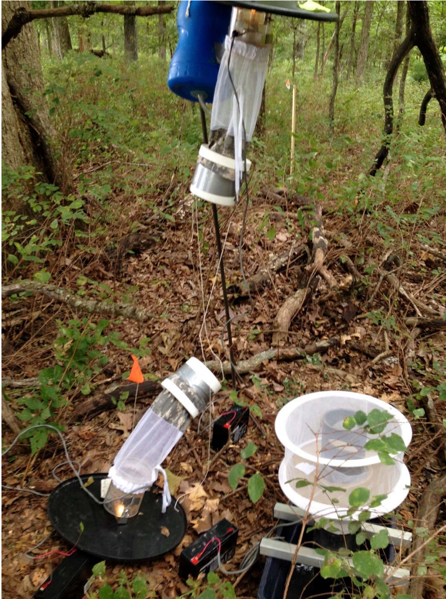
Figure 2.5, CDC miniature light trap with sand fly trap attached.
