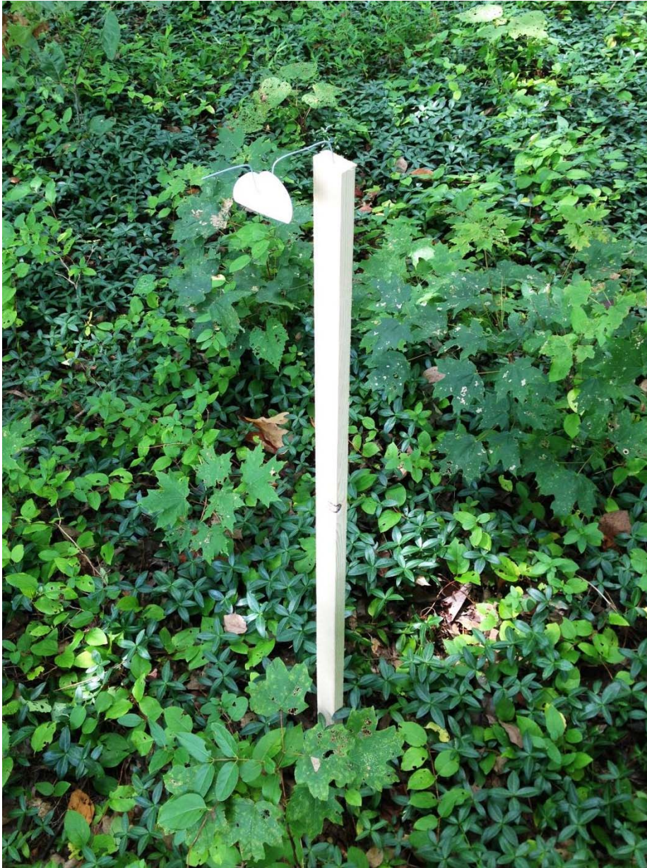
Figure 2.3, Treatment stake with wire and treatment filter paper.
