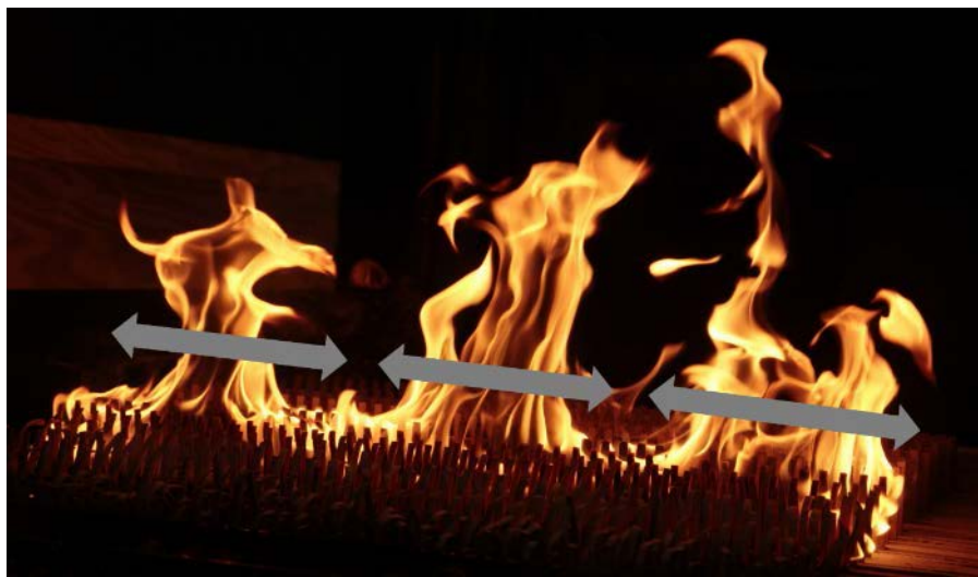
Figure 1.3 Peaks and valleys in propagating fire front [90].
