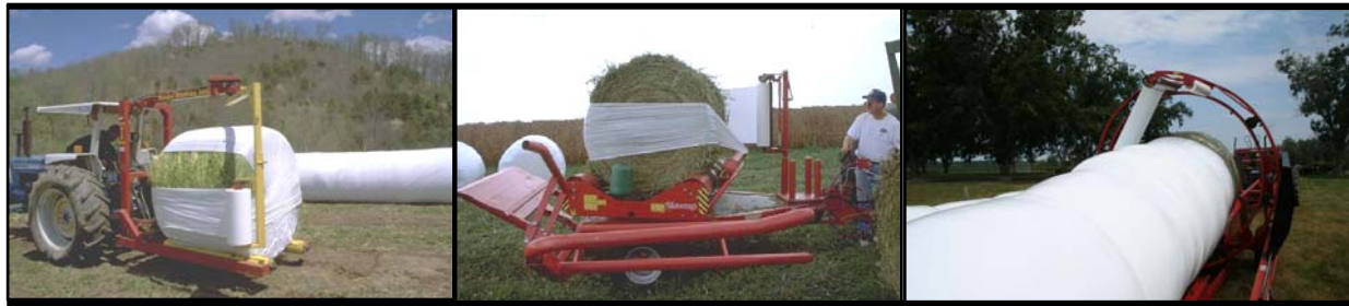
Figure 1. Examples of three basic categories of Balage wrappers: (L to R) individual bale wrapper on a 3-pt. hitch platform, individual bale wrapper on a trailer platform, and an in-line bale wrapper.
