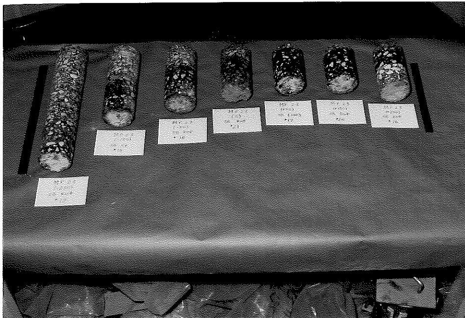
Figure B5. Field Cores Obtained from the Whitesburg Bypass at Approximate MP 2.3 (Section No. 8).
