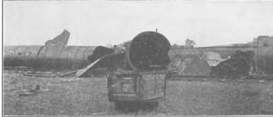
Figure 2.2 Altofts Experimental Gallery After Explosion of Dust Occupying 450 Linear Feet of Gallery, August 11, 1908 [Rice et al. 1911].
