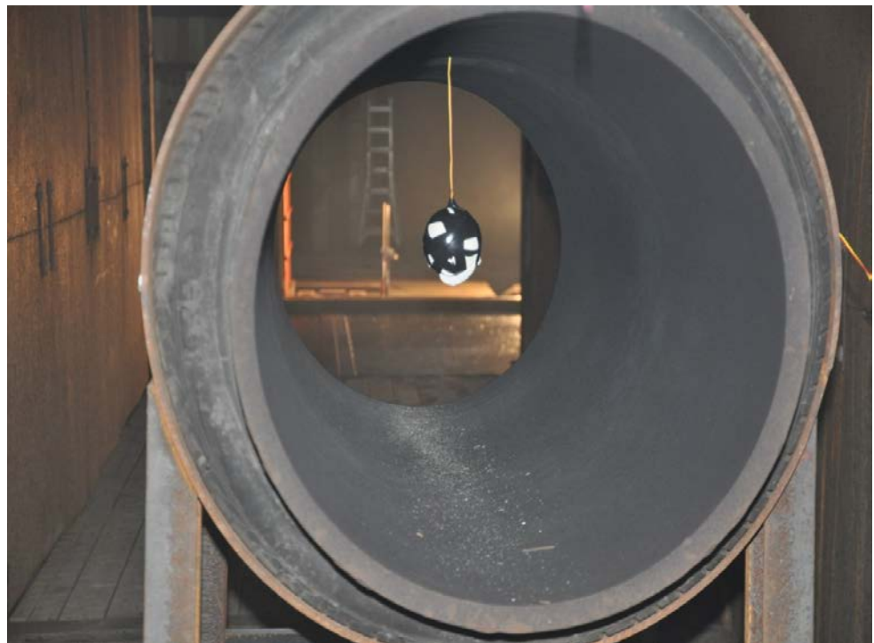
Figure 5.4 Explosive charge installed in shock tube
