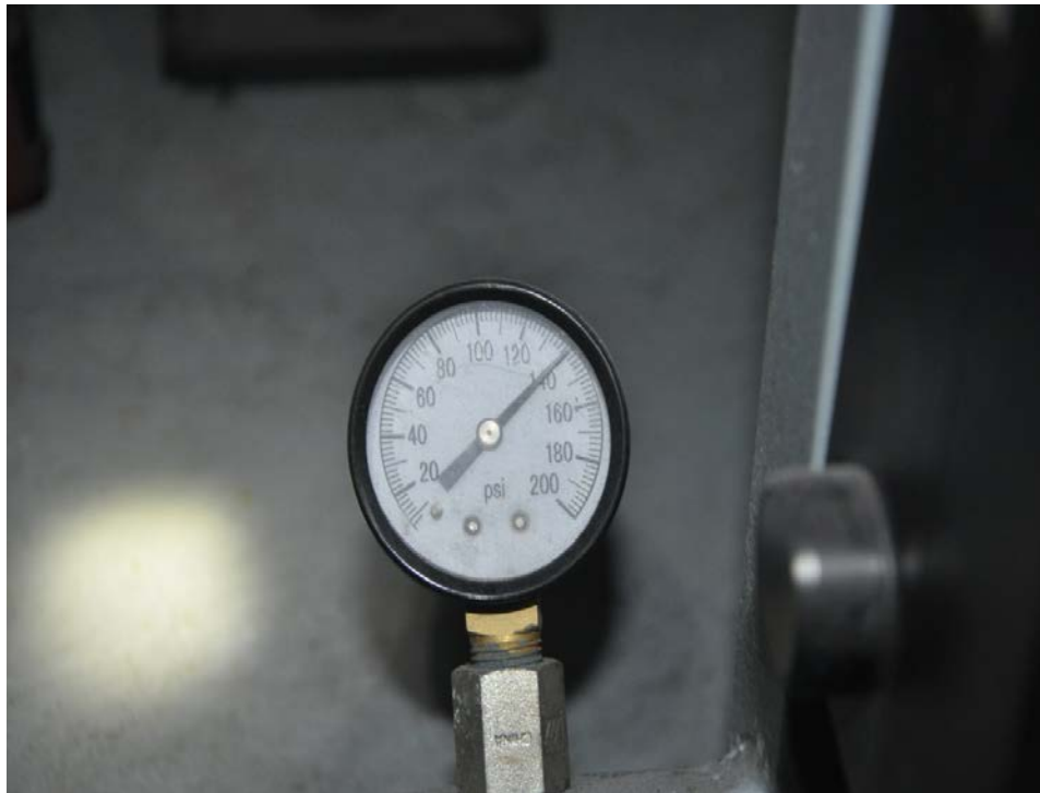
Figure 3.9 Pressure reservoir filled to 140 PSI
