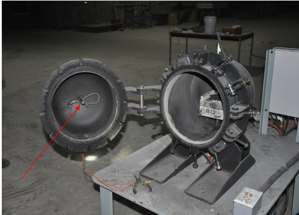
Figure 3.7 5kJ Sobbe igniter installed in chamber
