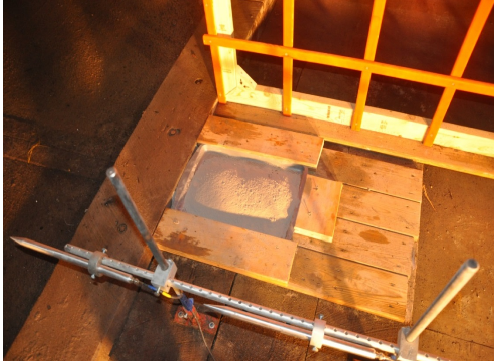
Figure 5.3 Large rock dust sample installed
