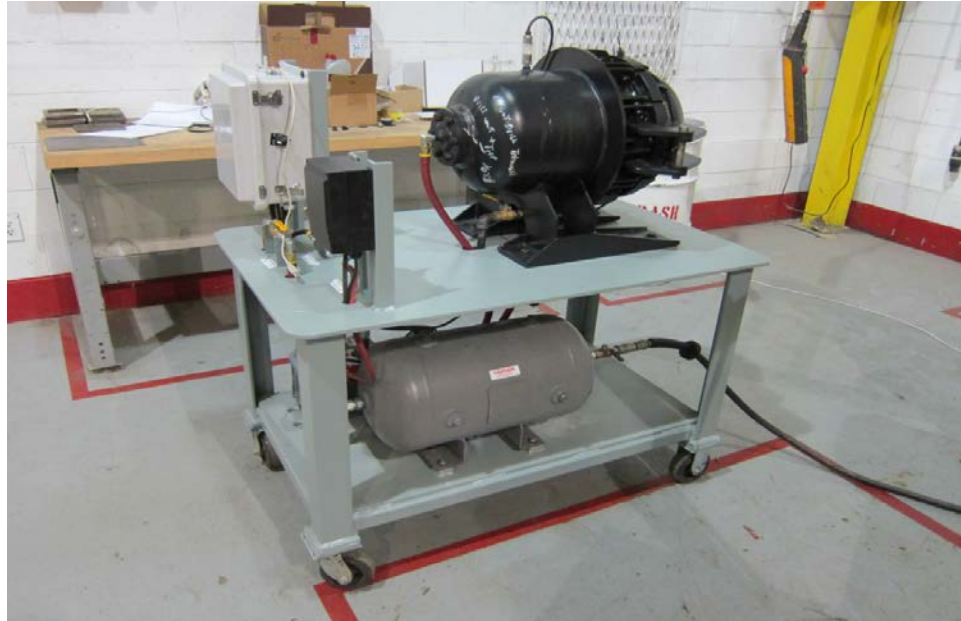
Figure 3.4 38 L Explosive Chamber
