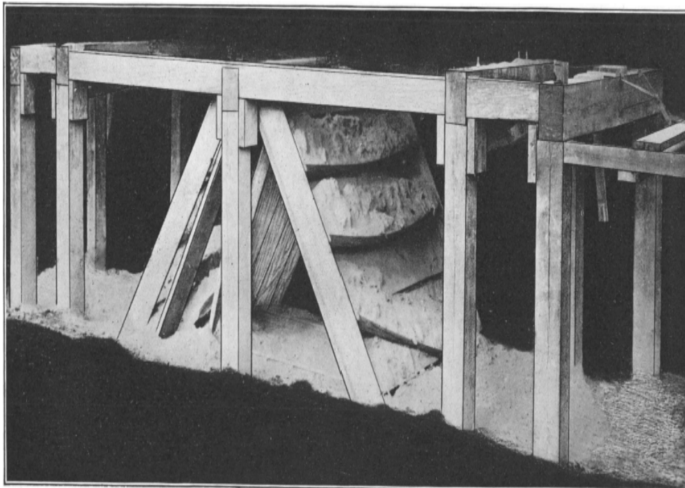
Figure 2.7 V-Trough Barrier Installed in Experimental Mine [Rice et al. 1922].
