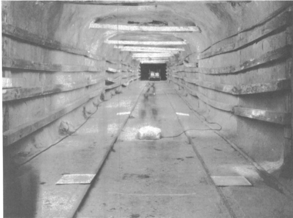
Figure 2.9 View of Mine Entry Before Rock Dusting by Aid of Permissible Explosives [Hartmann et al. 1950].
