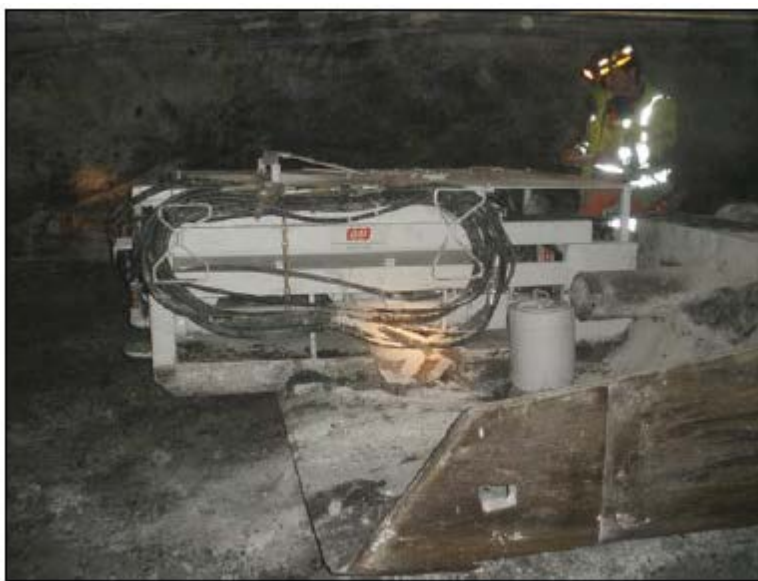
Figure 2.1 Rock Dust Machine Example [Pinkley et al. 2012]
