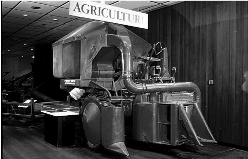
Figure 10. Old Red, a 1943 International Harvester cotton picker, one of the first successful models. (National Museum of American History, a gift of Producers Cotton Oil Company)
