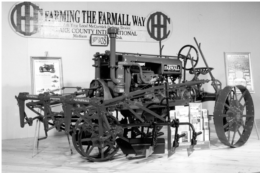
Figure 6. 1928 Farmall with attached two-row cultivator. (South Dakota State Agriculture Heritage Museum Photograph Archive)
