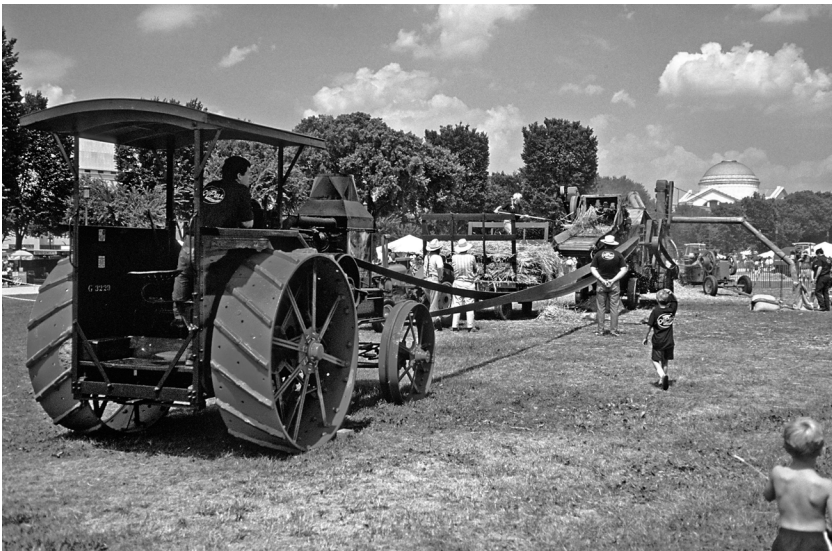
Figure 3. A restored Rumely Oil Pull steam tractor powering a threshing machine. (National Museum of American History)
