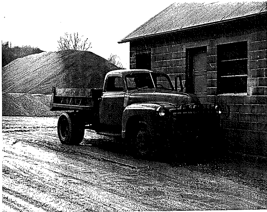
Fig. 3. At all aggregate sources the truck was weighed empty and full on the same scale in order to get the unit weight of the aggregates and also eliminate effects of differences among scales,
