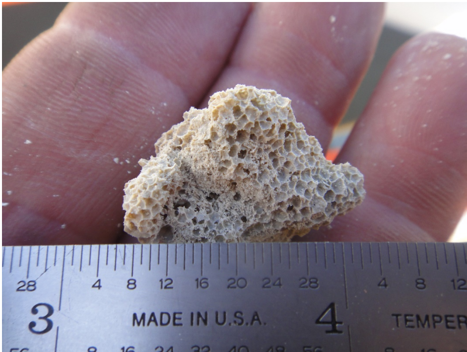
Figure 89. A Porous Grout Sample Extracted from A Void in Connection Sleeve C19D.
