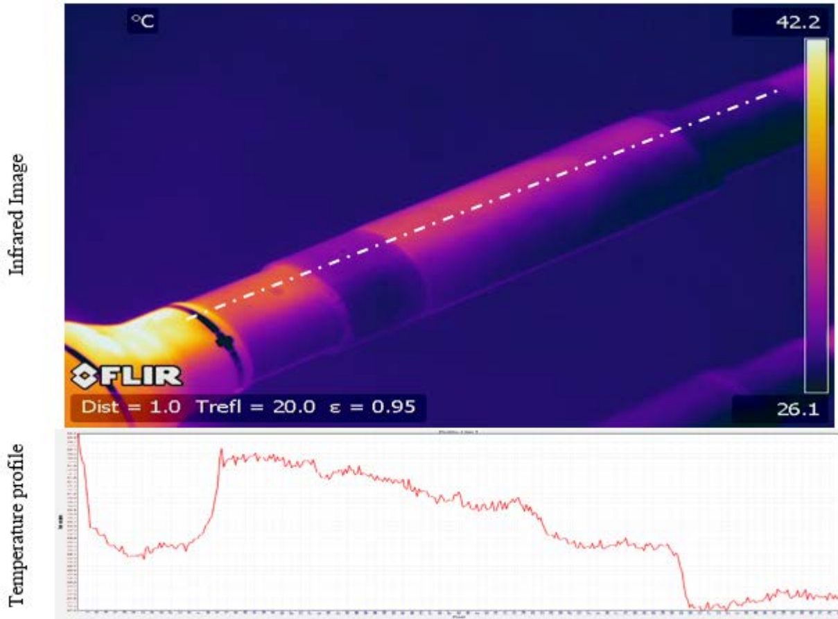
Figure 31. Infrared Image of the Tower Anchorage Connection Sleeve Pipe Section for Cable B3D and Thermal Profile for the Dashed Line Shown in the Infrared Image (Op. Cit. 10, p. 24).
