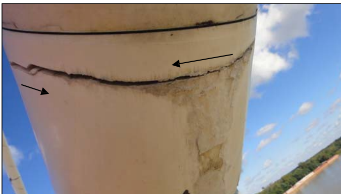
Figure 28: B20U: Top Coupler Crack at Weld Nipple Hole Propagating into and around the Reducer (Top 4 photographs) & Crack at Bottom Coupler (Bottom 2 photographs)
