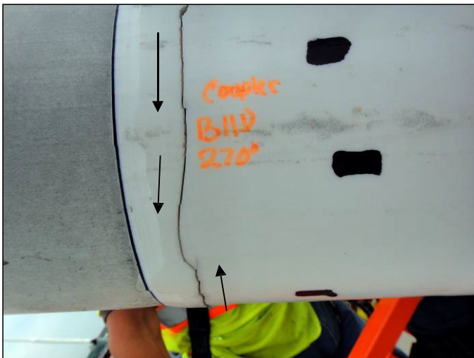
Figure 13: B11D : Reducer Crack at Coupler Hole Used For Electro-Fusion Weld
