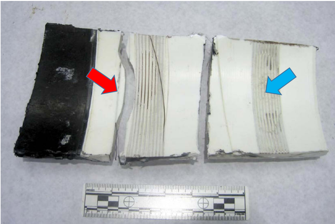
Figure 14. Extracted Coupon (Inner View). Note Fracture Face (Red Arrow) and Lack of Fusion Area in Electrofusion Weld (Blue Arrow).
