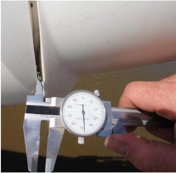
Figure 50. (a) Measuring Large Crack Opening with a Vernier Caliper; (b) Measuring Small Crack Opening with a Comparator Gage.
