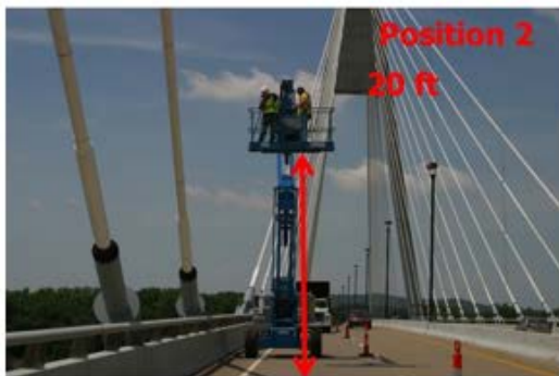
Figure 25. Use of a Man Lift to Take Thermal Images of the Stay Cable Piping at Various Heights above Deck Level (Op. Cit. 10, p. 11).
