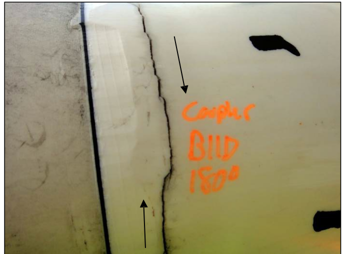
Figure 13: B11D : Reducer Crack at Coupler Hole Used For Electro-Fusion Weld
