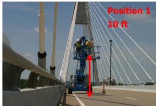
Figure 24. Measuring Grout Voids Based upon GPR and Sounding Tests.
