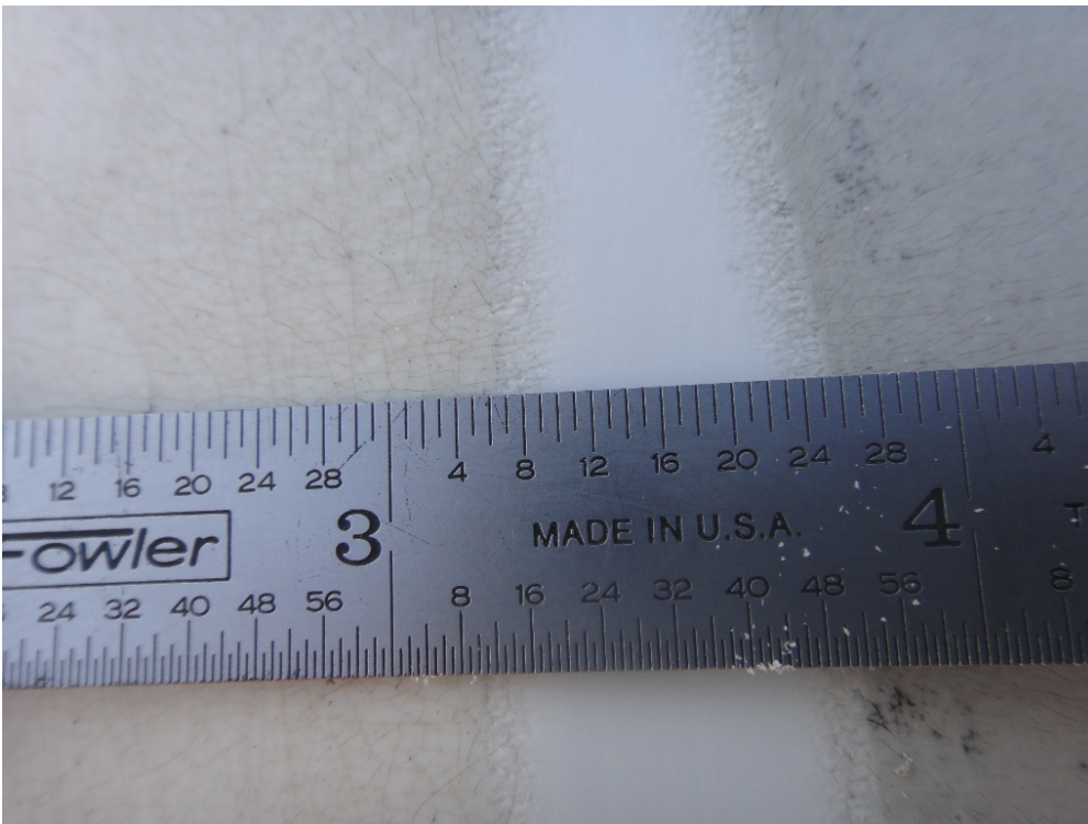
Figure 83. Surface of Coextruded HDPE Piping after Taking a Surface Scrape Sample.
