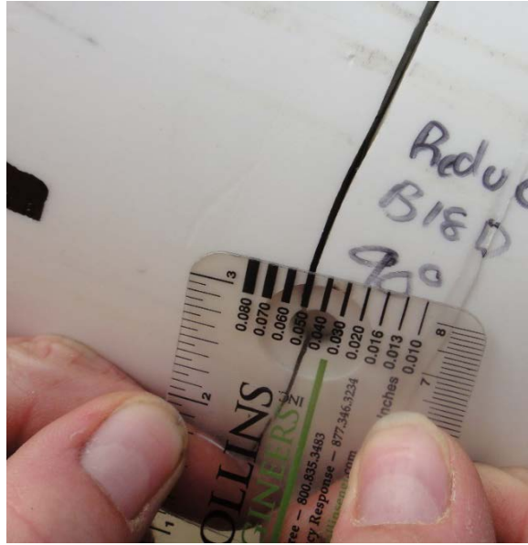
Figure 50. (a) Measuring Large Crack Opening with a Vernier Caliper; (b) Measuring Small Crack Opening with a Comparator Gage.
