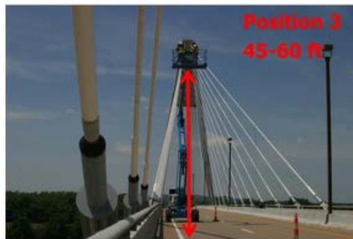
Figure 25. Use of a Man Lift to Take Thermal Images of the Stay Cable Piping at Various Heights above Deck Level (Op. Cit. 10, p. 11).
