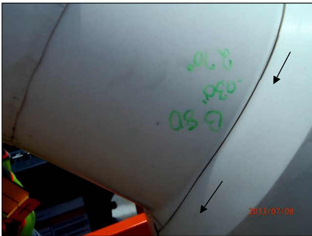
Figure 10: B8D: Reducer Crack at Notch Located at Diameter Transition
