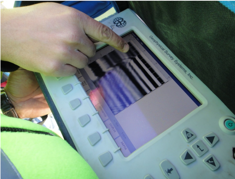
Figure 20. Grout Void Indication on GPR Monitor Screen.
