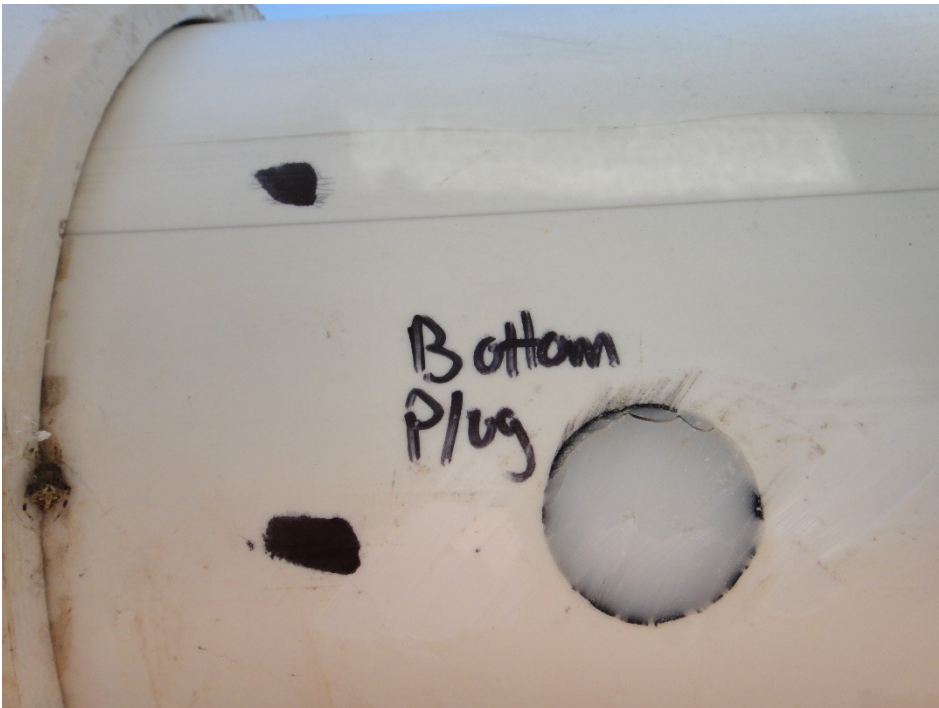
Figure 66. Grout Plug with Minor Cracking.
