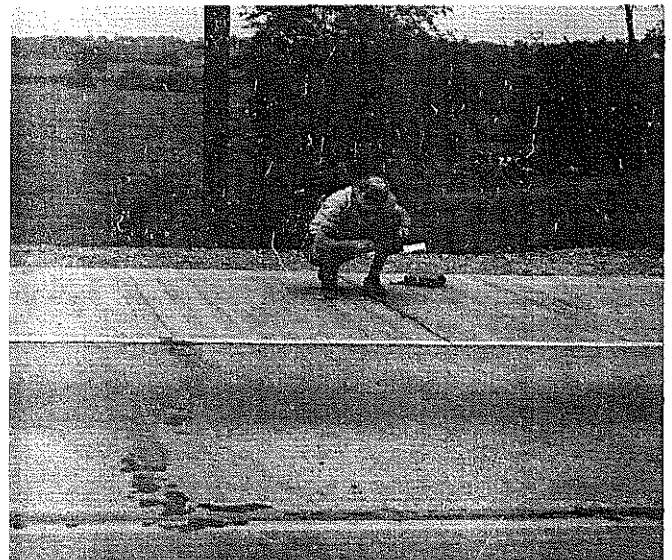
Fig. 26. Making width measurements over Joint No. 2 at Station 245,450 in June, 1951. At this time the truck lanes had been in service about 8 months, and there was no apparent difference in the condition of the standard and the aluminum joints, nor any difference in the condition of the concrete about the two types of joints.
