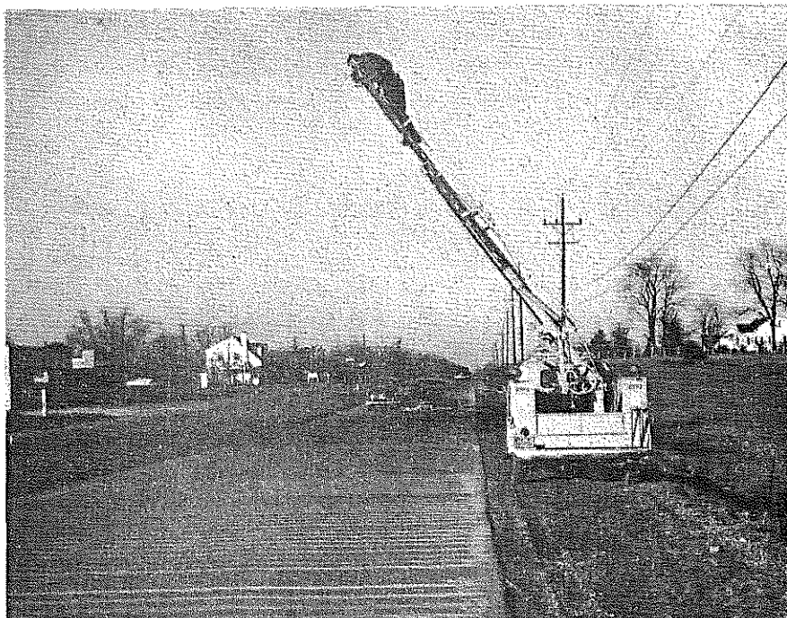
Photograph illustrating method of photographing stripes for preparing comparison mosaics. This method seemed to be the most practical for showing such a large number of stripes. Duplicate pictures were made in daylight with diffuse light and at night with flash. In this case, flash photography simulates the small divergence angle of night-time viewing conditions.
