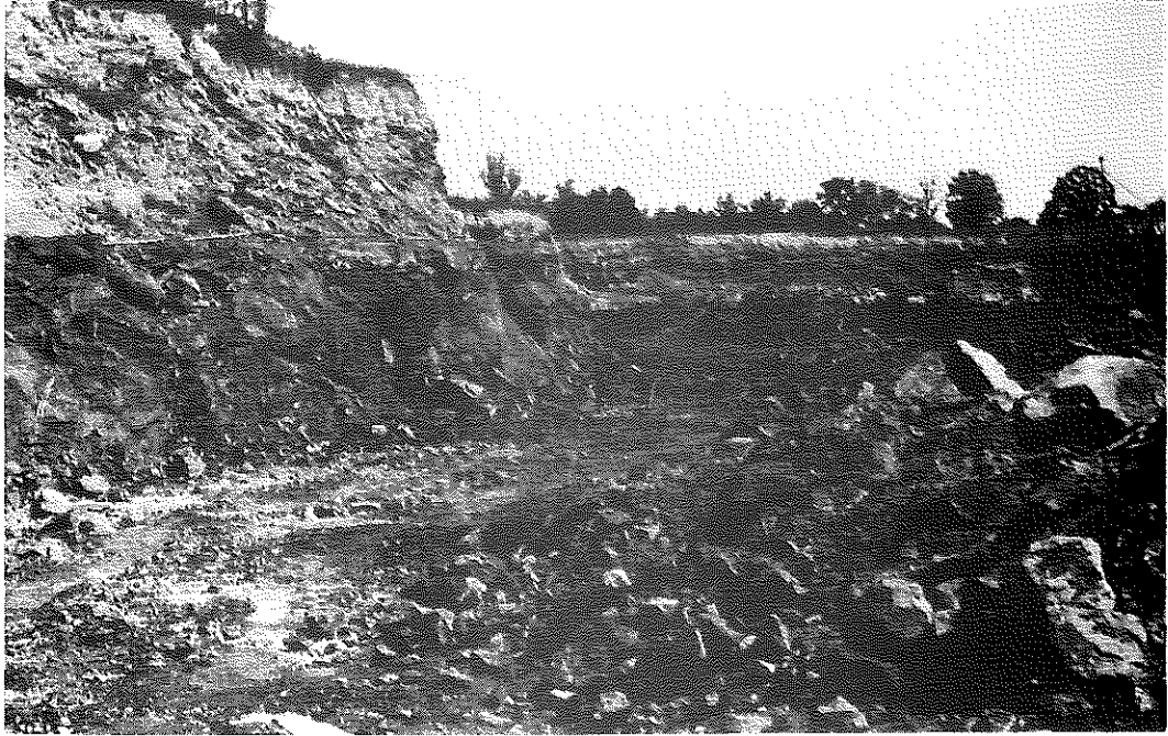
FIG. 6: West Face of the Black Gold Quarry. Usable rock is shown under the pipe line at the left of picture.
