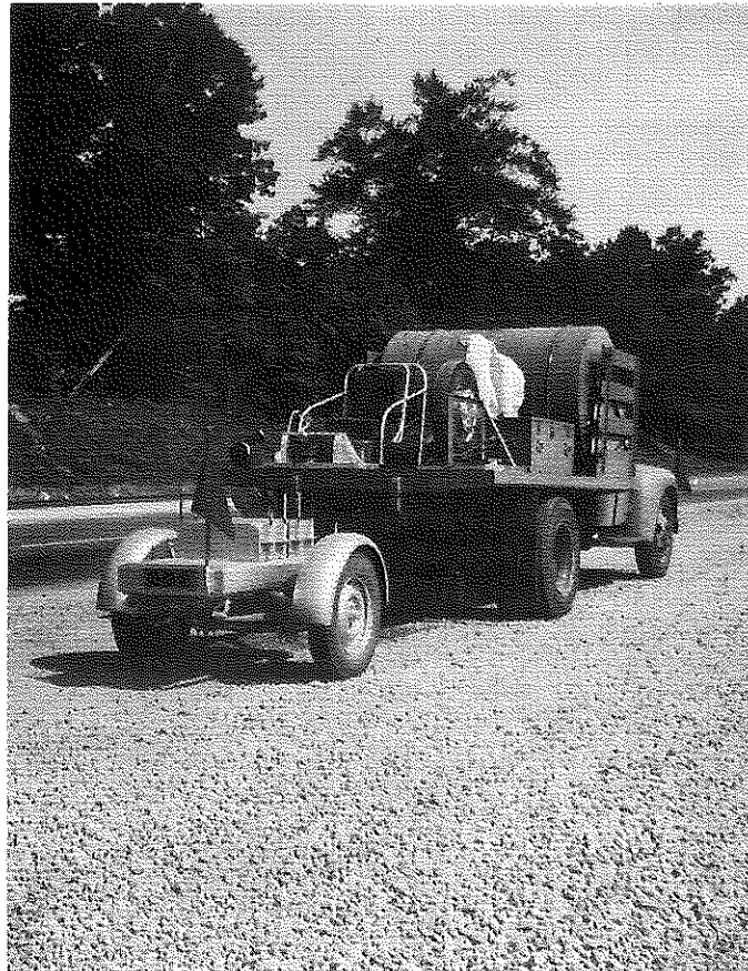
Fig. IV-a: Skid-test Equipment used by the Tennessee Highway Research Program in Cooperative Tests on Kentucky Roads.
