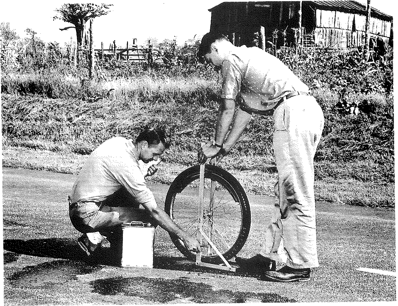
Fig. 3. Slipperiness Tester, Patterned after the National Crushed Stone Association's Goldbeck-Wheel; Consisting of a Weighted Bicycle Wheel; Adaptation of a Pendulum.
