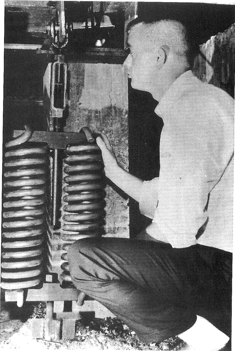
Figure 6. Coil Spring Preload Device.
