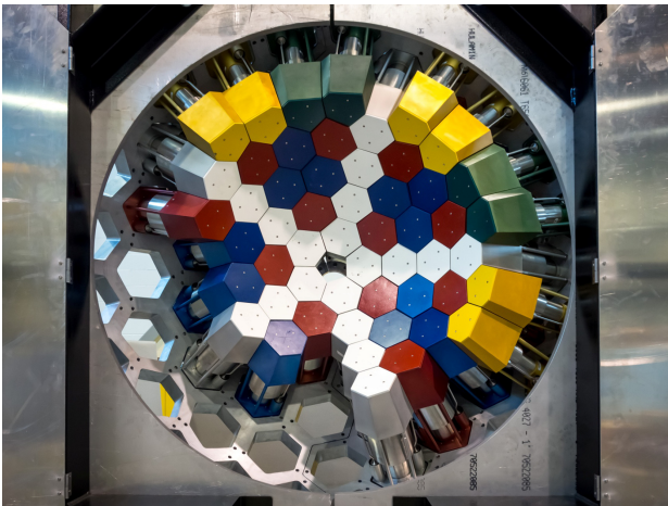
Figure 2. Photo of DESCANT detectors mounted on an assembly stand. The different colors of the detectors denote their different shapes.
