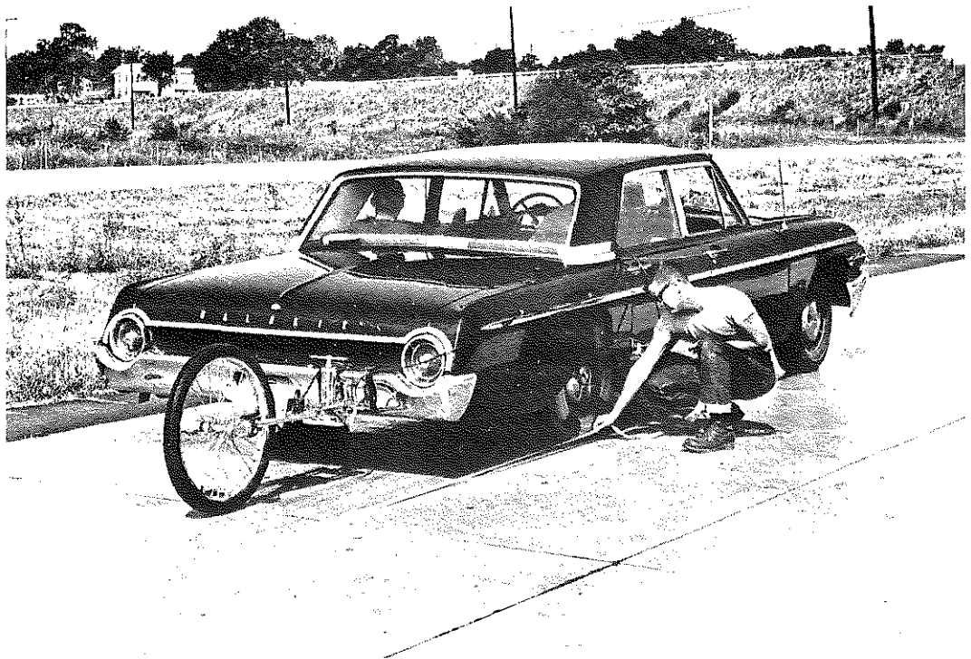
Figure 4. Test Vehicle During Measurement of "Observed" Stopping Distance.
