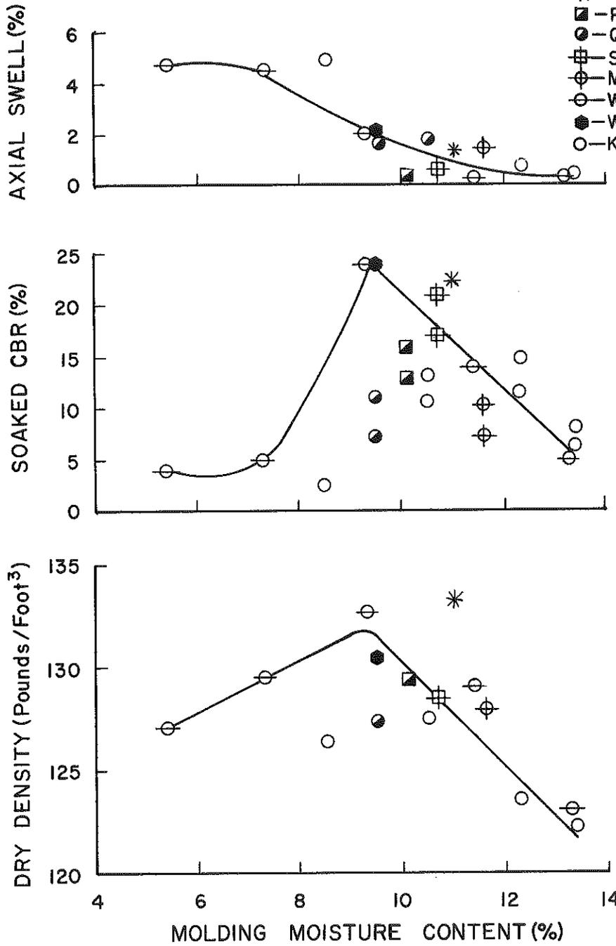
Figure 11. CBR Data, AASHTO Soil Sample, Method 4.
