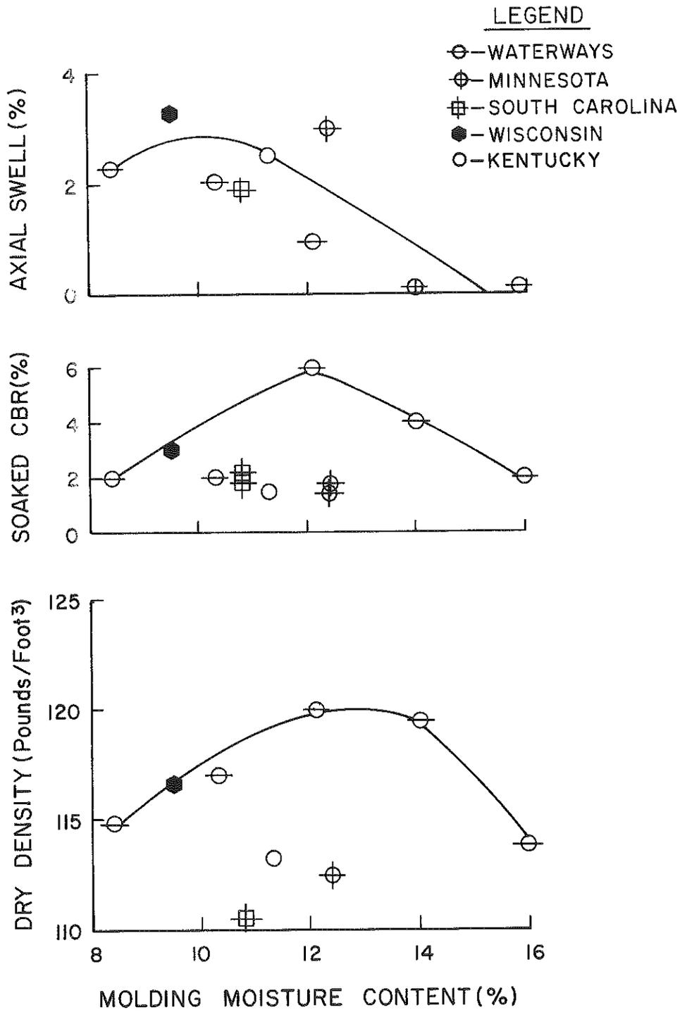
Figure 13. CBR Data, AASHTO Soil Sample, Method 4 (12 blows/layer).
