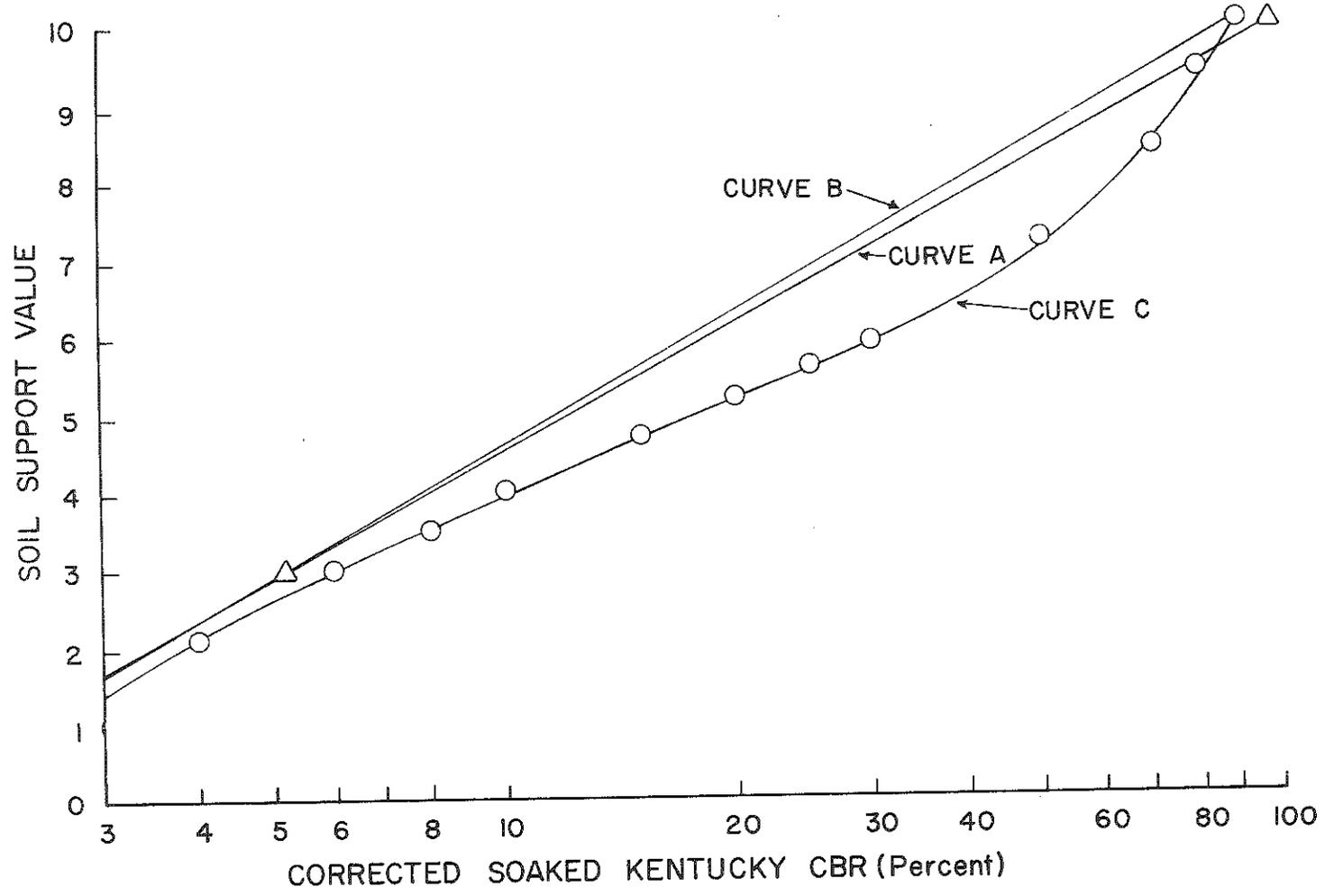
Figure 15. Soil Support Value - Corrected Soaked Kentucky CBR Correlation Curves A, B, and C.
