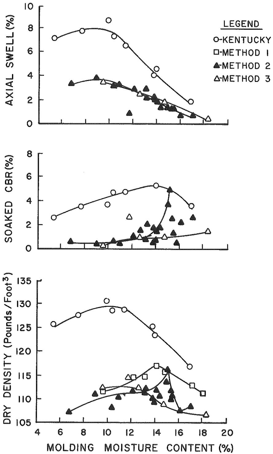
Figure 2. CBR Data, AASHTO Road Test Soil Sample.
