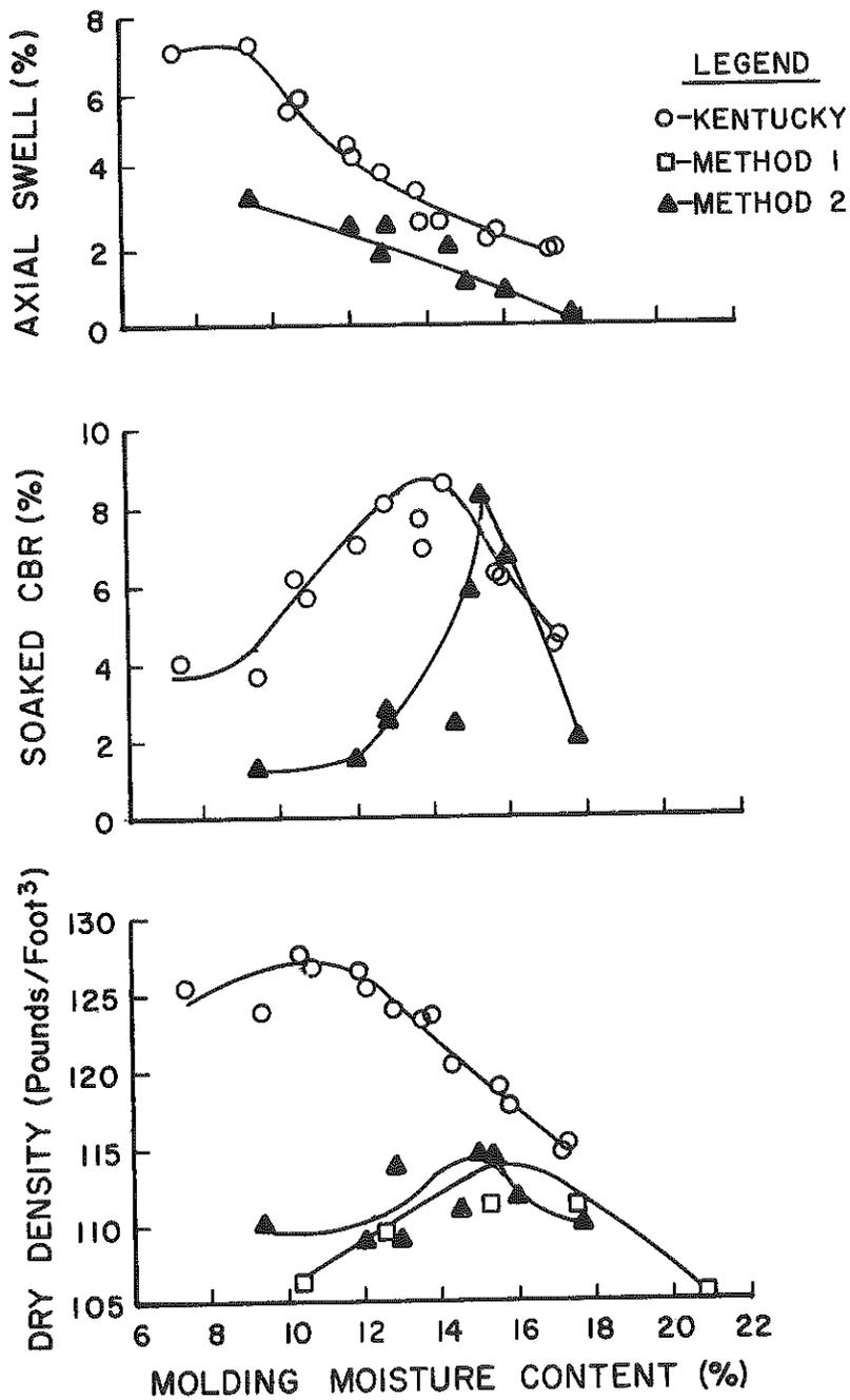
Figure 3. CBR Data, Soil Sample From State of Ohio.
