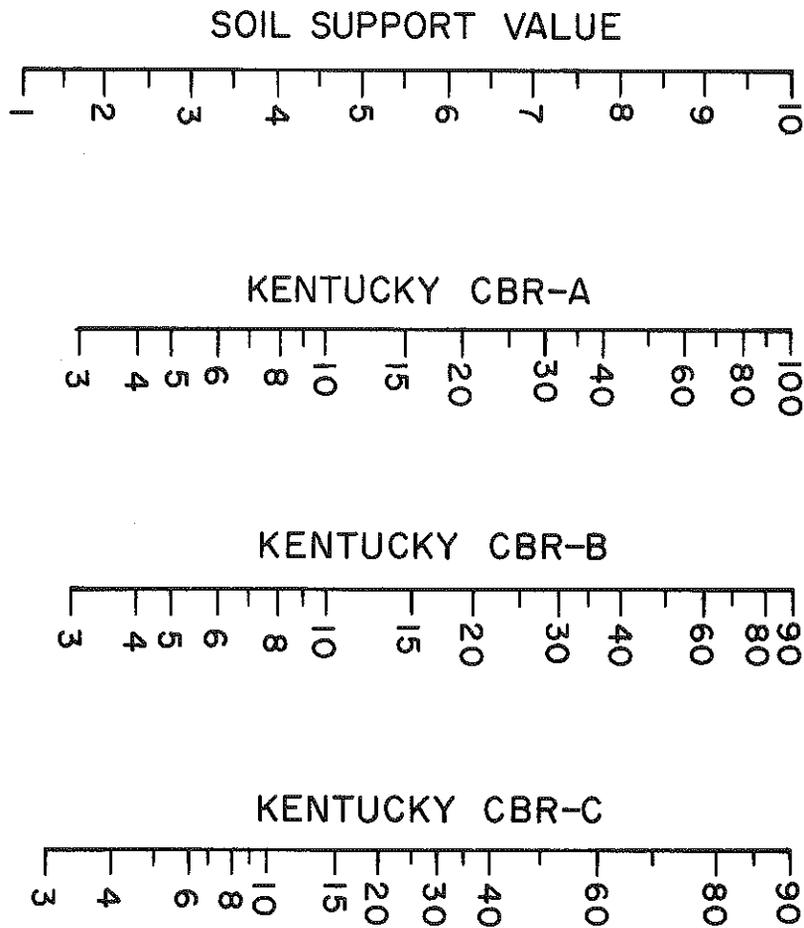
Figure 17. Soil Support Value - Kentucky CBR Nomographs A, B, and C.
