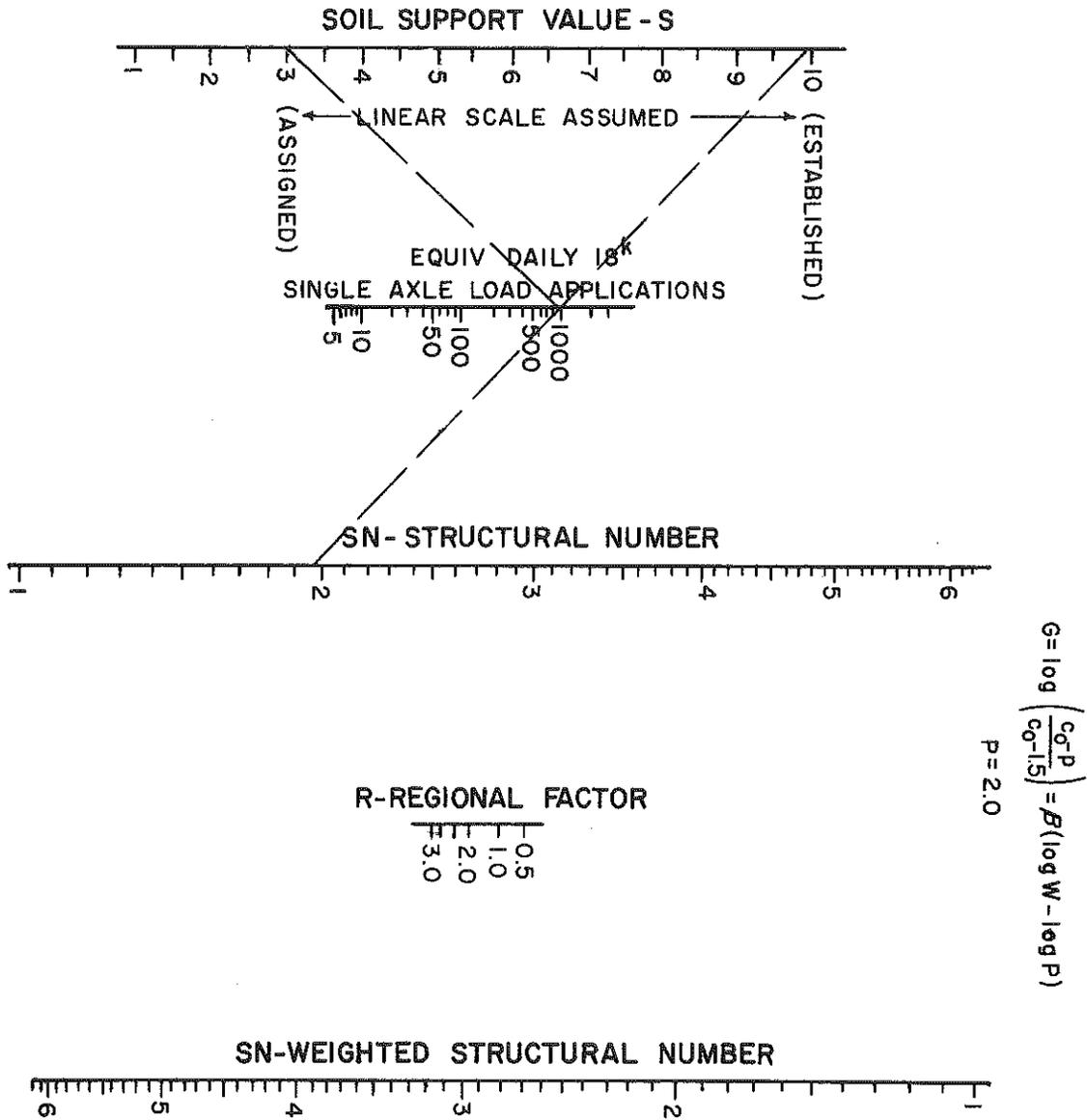
Figure 1. AASHO Flexible Pavement Design Chart ( $P_t = 2.0$ ).
