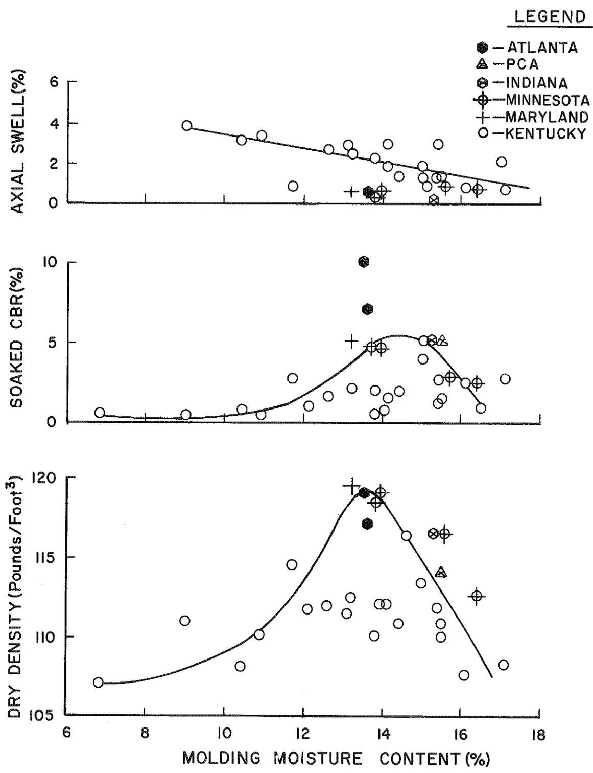
Figure 10. CBR Data, AASHO Soil Sample, Method 2.
