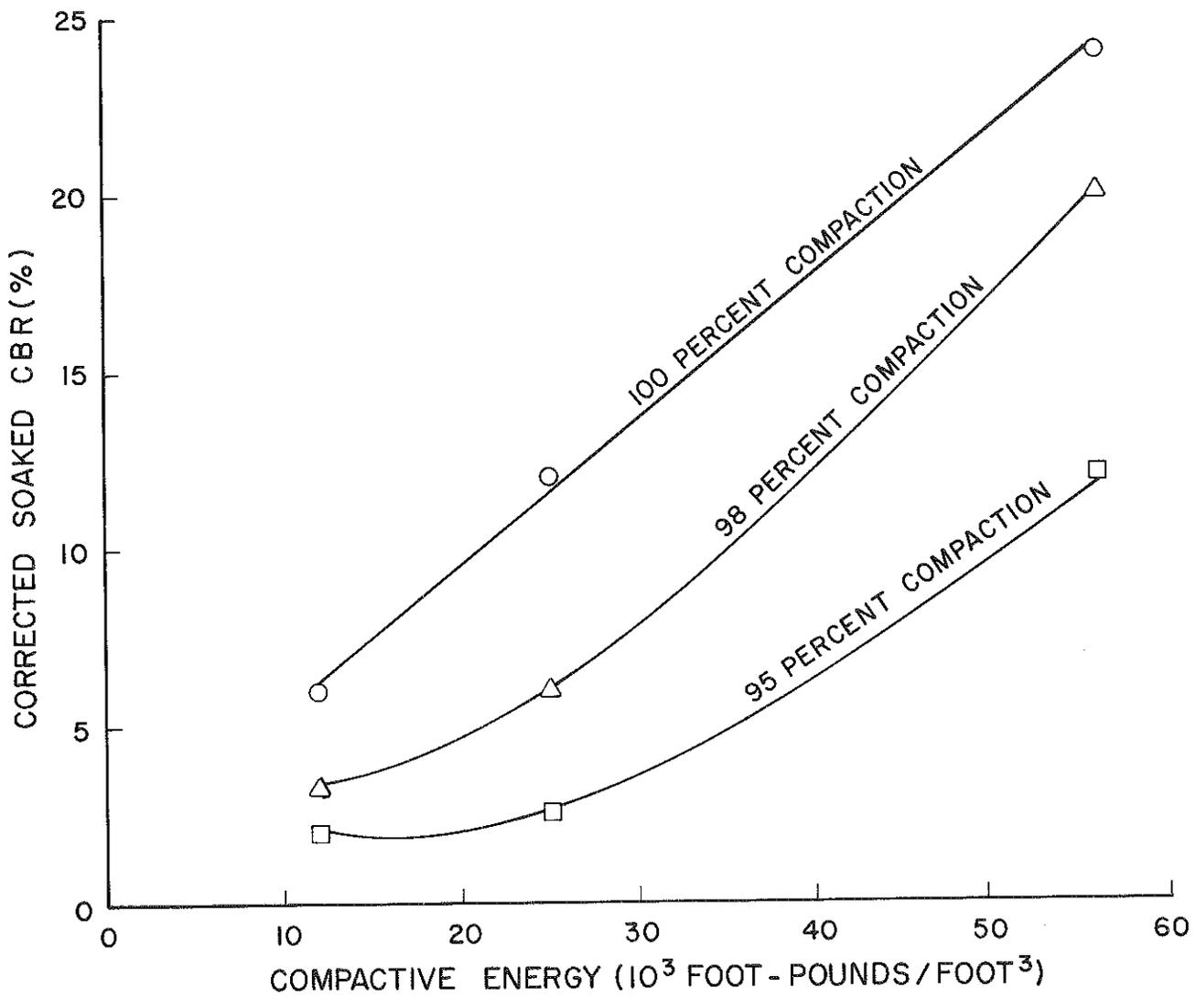
Figure 14. Corrected Soaked CBR - Compactive Energy Curves, AASHO Soil Sample.
