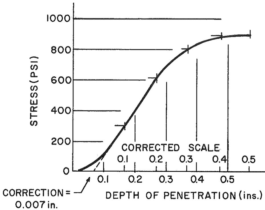
Figure 18. Example of Suggested Method for Correcting Stress-penetration Curves to Obtain True Values of Stress and Depth of Penetration to be Used in Computing CBR's.
