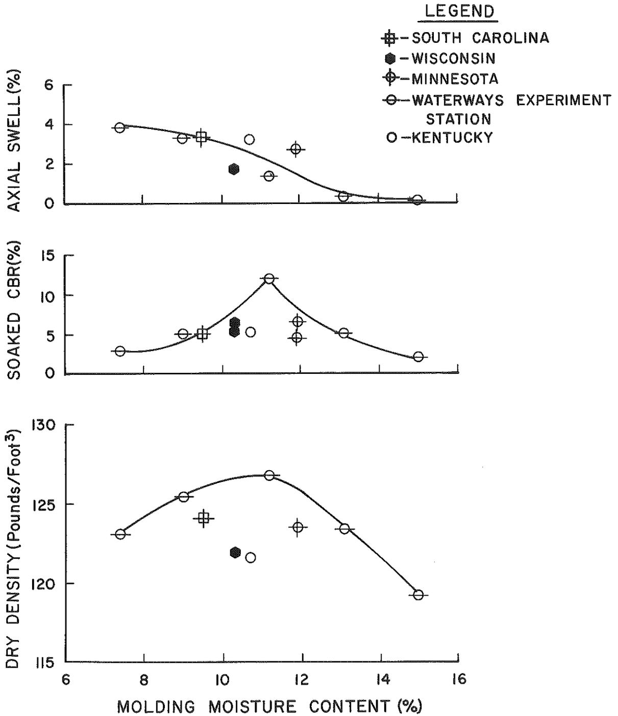
Figure 12. CBR Data, AASHO Soil Sample, Method 4 (25 blows/layer)
