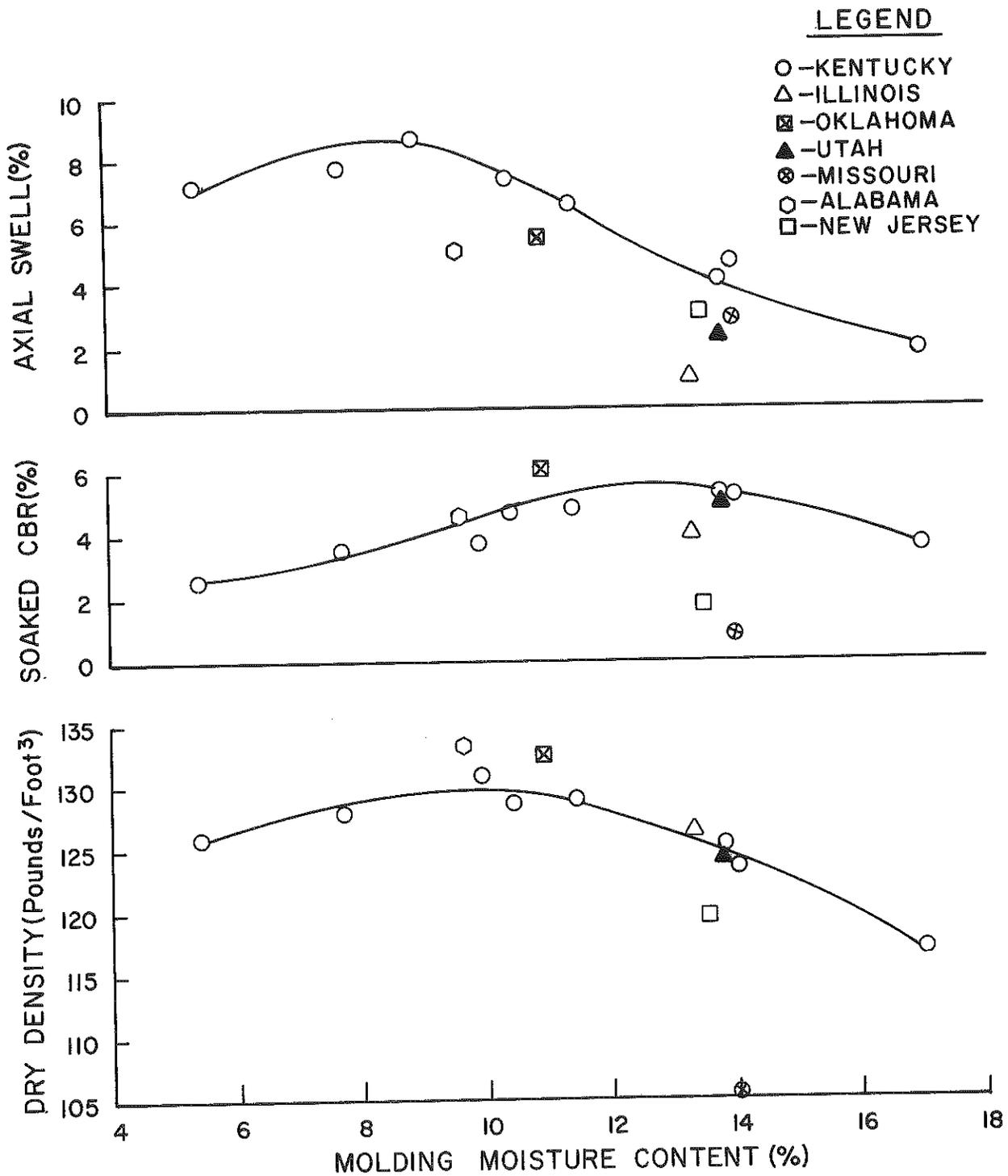
Figure 9. CBR Data, AASHO Soil Sample, Static Compaction.
