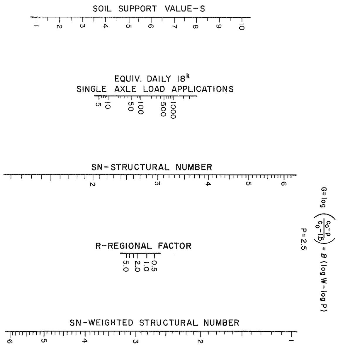
Figure 20. AASHO Flexible Pavement Design Chart ( $P_T = 2.5$ ).
