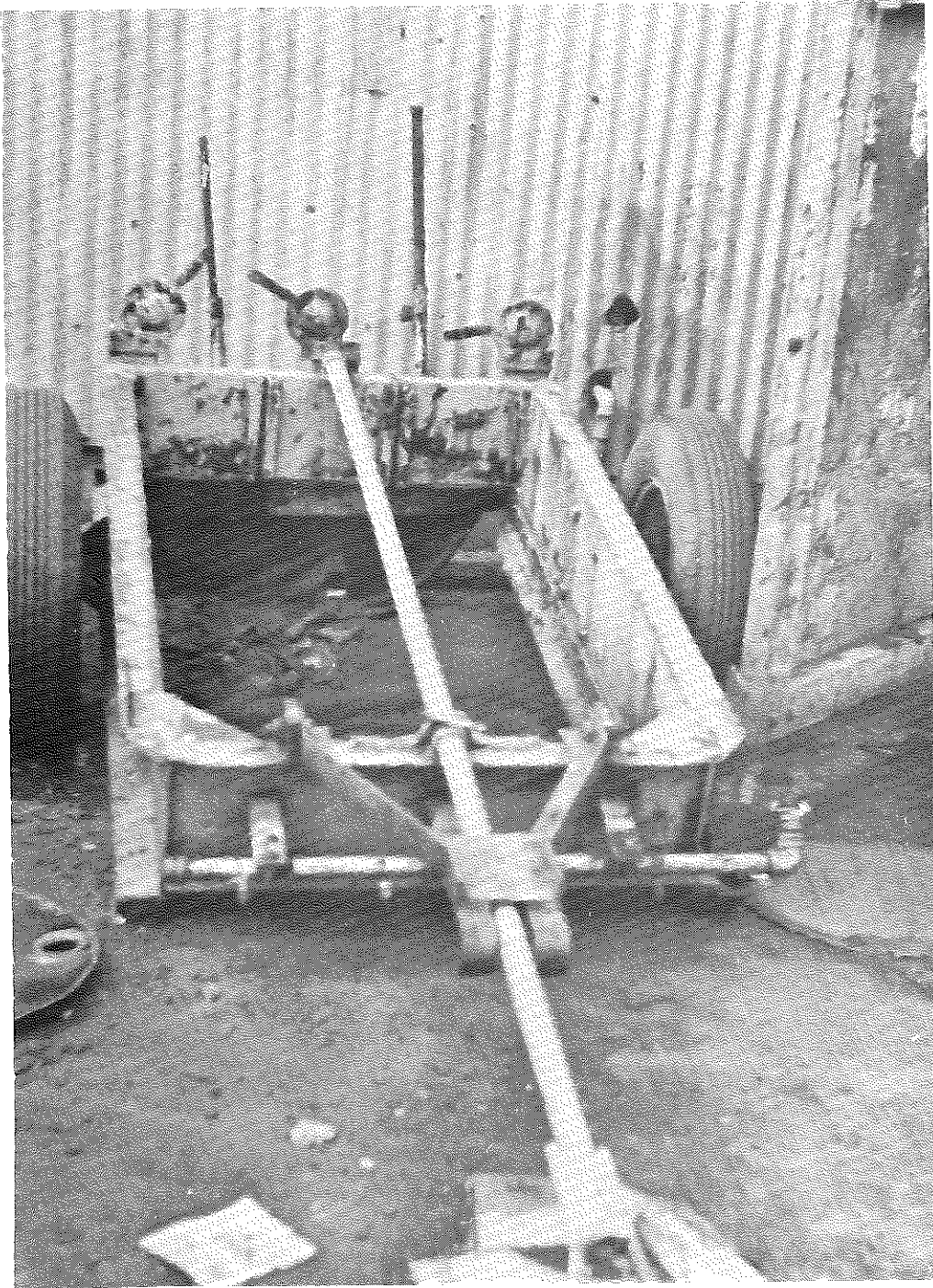
Figure 31. Spreader box constructed by Maintenance forces for sealing bituminous shoulders.
