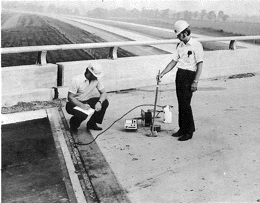
Figure 8. Corrosion Potential Testing Apparatus.
