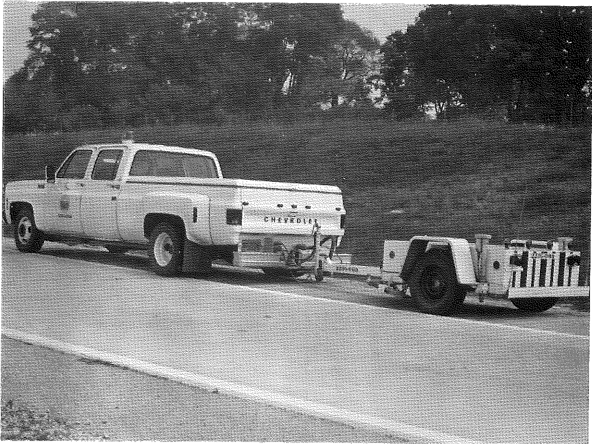
Figure 6. Pavement Friction Tester (Model 1270) (Survey Type).
