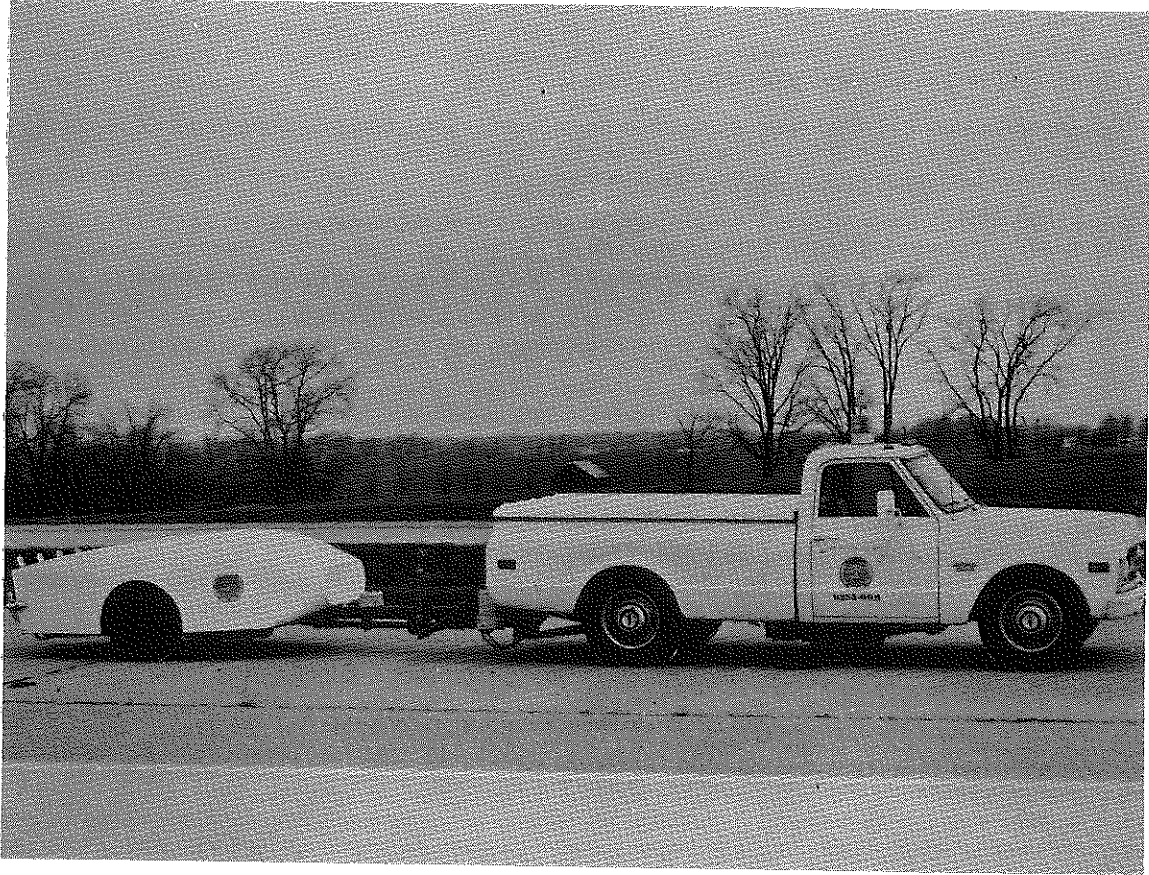
Figure 3. Surface Dynamic Pavement Friction Tester (Model 965A).
