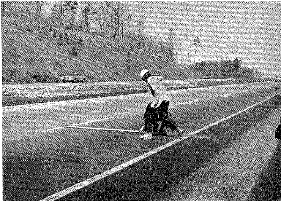
Figure 32. Tendency toward Rutting in Asphaltic Concrete Pavements Carrying Heavy Traffic.
