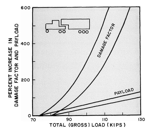
Figure 7. Increases in Damage Factor and Payload as Gross Vehicle Weight Increases for a Six-Axle Combination Tractor-Trailer Truck.
