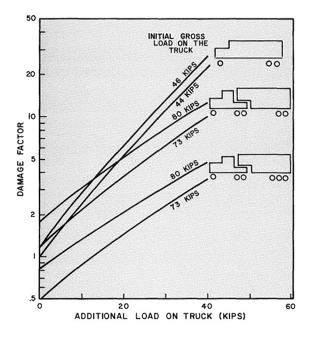
Figure 4. Increase in Damage Factor for Selected Vehicles as Load on Truck Is Increased.
