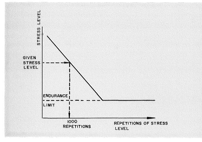
Figure 2. Idealized Stress-Repetitions (S-N) Curve.
