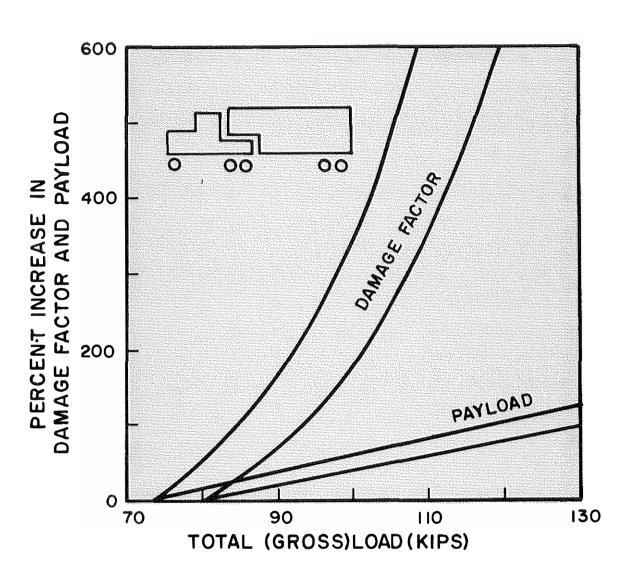
Figure 6. Increases in Damage Factor and Payload as Gross Vehicle Weight Increases for a Five-Axle Combination Tractor-Trailer Truck.
