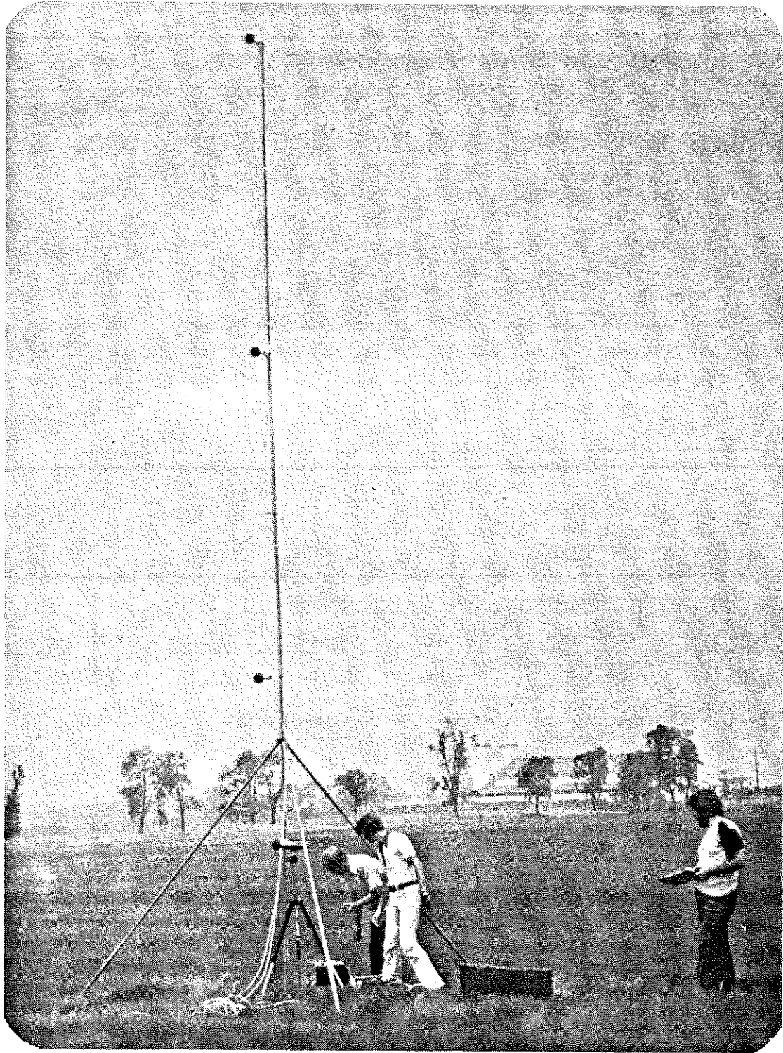
Figure 2. Photograph of Setup Used to Collect Data Simultaneously at Four Measurement Heights.
