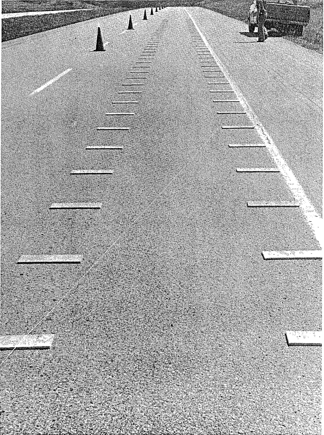
Figure 2. Test site with plywood used to simulate rumble strips.
