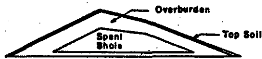
Figure 2. Unsymmetrical Configuration of Oil Shale Disposal Embankment to Control Surface Drainage (not to scale).
