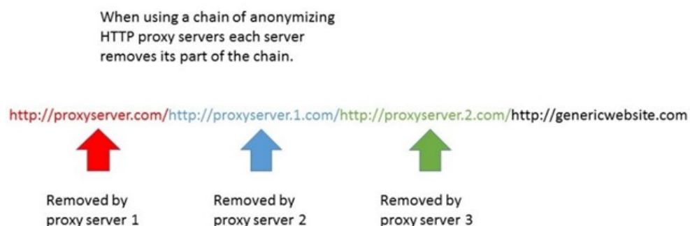
Figure 3. Rewebber chain constructed using three rewebbers
