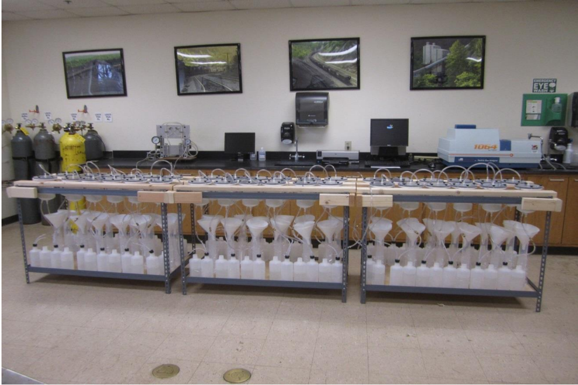
Figure 5.2. Column leaching tests set-up
