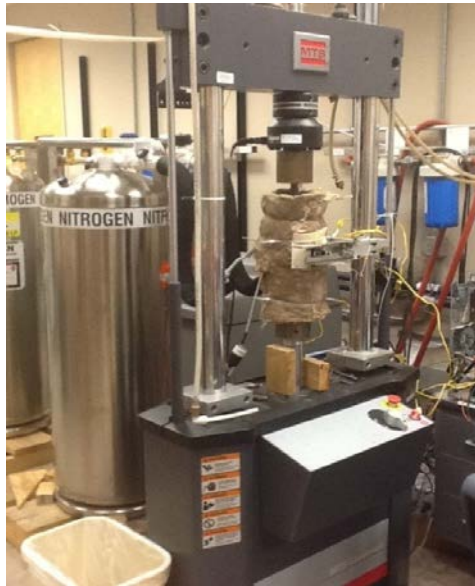
Figure 6.3 Shows the MTS setup used for testing mechanical behavior of CNT-SMP composites.
